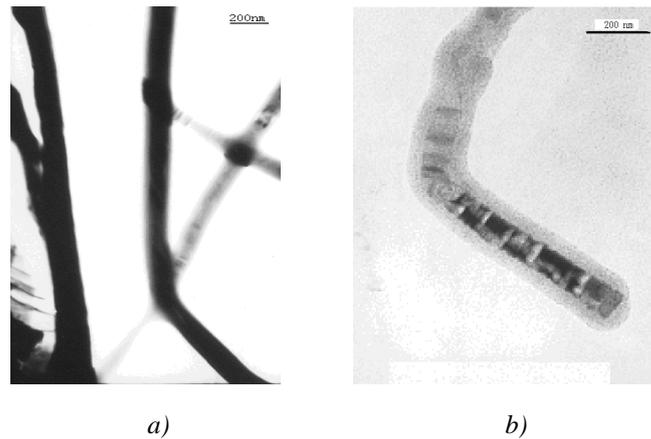
Fig. 2. TEM micrographs of silicon nitride nanowires(a, silicon nitride nanowires; b, growth of silicon nitride nanowire)
