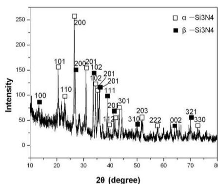
Fig. 1. X-ray diffraction spectrum of silicon nitride nanorods
