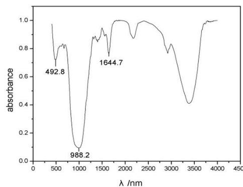
Fig.3. FTIR spectra of the silicon nitride nanowires
