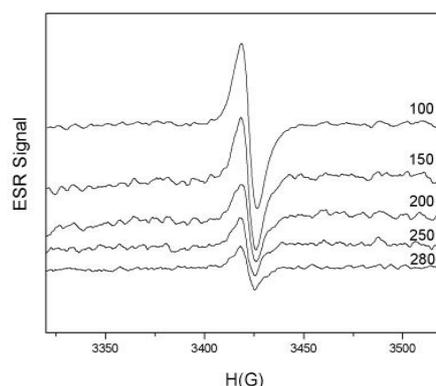
Fig.4 ESR curves of silicon nitride nanowires at different temperature
