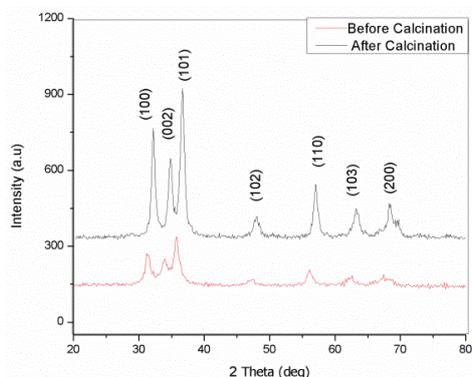
Fig. 1. XRD pattern of the as prepared and calcined ZnO nanoparticles
