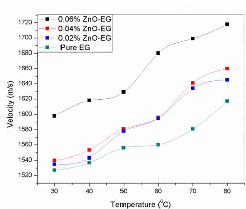
Fig.4. Ultrasonic velocity of base fluid and ZnO-Ethylene glycol nanofluid at low concentrations(0.02%,0.04% and 0.06%)
