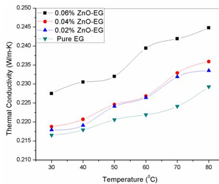
Fig.7. Thermal conductivity of base fluid and ZnO-Ethylene glycol nanofluid at low concentrations(0.02%,0.04% and 0.06%)
