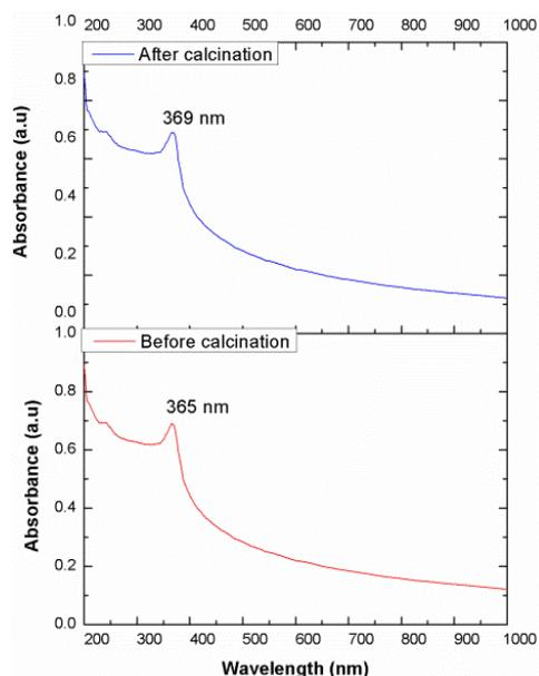
Fig. 2.a. Absorbance of the ZnO nanoparticles before and after calcinations
