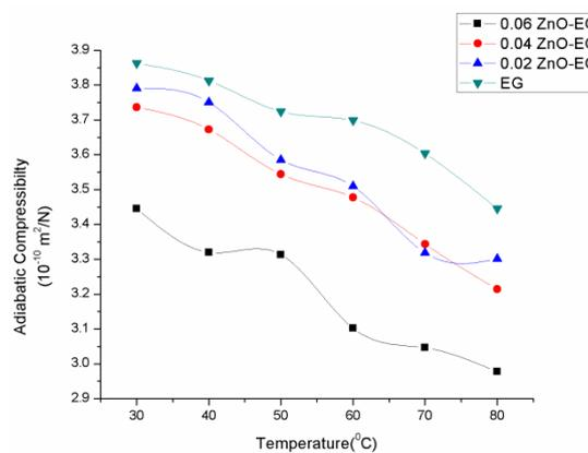
Fig.5. Adiabatic compressibility of base fluid and ZnO-Ethylene glycol nanofluid at low concentrations(0.02%,0.04% and 0.06%)
