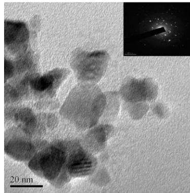
Fig.3. TEM analysis of pure ZnO nanoparticles
