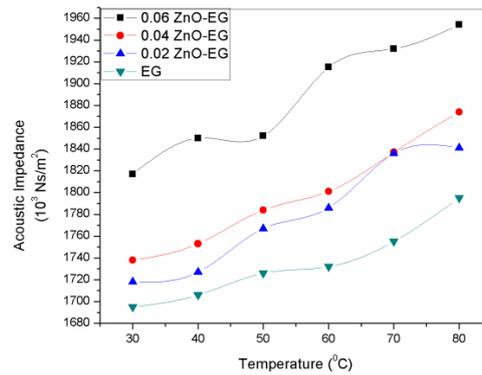
Fig.6. Acoustic impedance of base fluid and ZnO-Ethylene glycol nanofluid at low concentrations(0.02%,0.04% and 0.06%)
