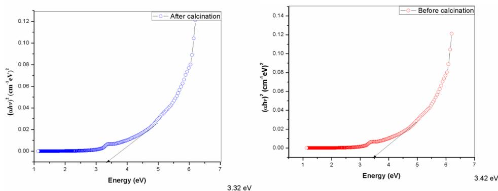
Fig. 2.b. Absorbance of the ZnO nanoparticles before and after calcinations
