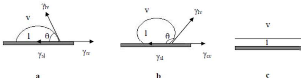
Fig. 1 - Contact angle between a liquid (l) and a flat solid surface (s): (a) and (b) correspond to partial wetting ( $\theta > 0$ ) and (c) corresponds to complete wetting ( $\theta = 0$ ).
