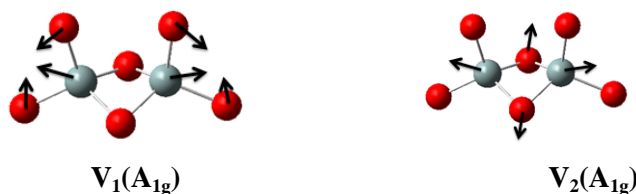
Fig.5. Schematic illustration of the main vibrational modes of \text{ES-Si}_2\text{S}_6 and \text{ES-Si}_2\text{Se}_6
