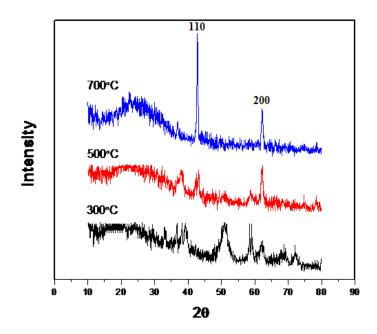
Fig 1. XRD spectrum of MgO nanoparticles at three calcinating temperature.
