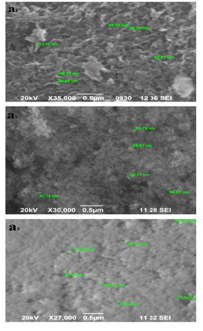
Fig 2.SEM images of MgO nanoparticles at different calcinating temperature  $a_1 = 300^{\circ}$ C,  $a_2 = 500^{\circ}$ C,  $a_3 = 700^{\circ}$ C.
