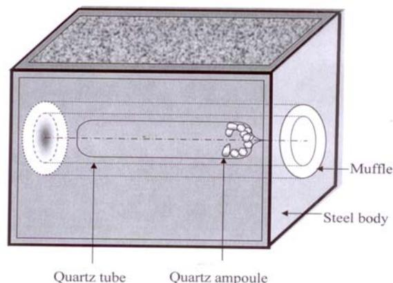
Fig. 1. The dual zone horizontal furnace with co-axially loaded ampoule.
