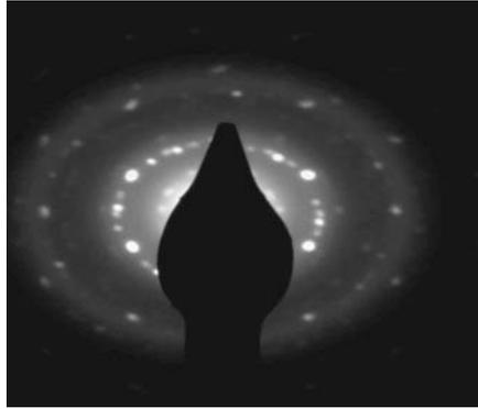
Fig. 6. Electron diffraction photograph of  $\text{SnSe}_{0.5}\text{Te}_{0.5}$  single crystal.
