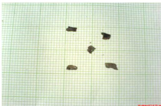
Fig. 4. Photograph of grown  $\text{SnSe}_{0.5}\text{Te}_{0.5}$  single crystals.
