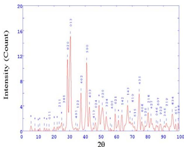
Fig. 5. X- ray diffractogram of  $\text{SnSe}_{0.5}\text{Te}_{0.5}$  crystal grown by direct vapour transport technique.
