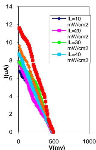
Fig. 9. Variation of photocurrent versus photovoltage for different illumination of light.
