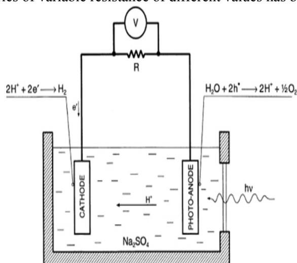
Fig. 3. Schematic diagram of PEC solar cell.
