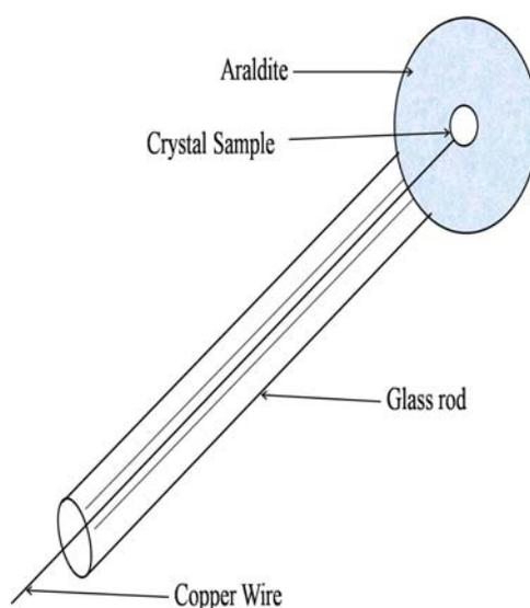
Fig. 2. The semiconductor electrode for PEC solar cell.
