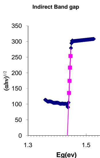
Fig. 8.  $(\alpha h\nu)^{1/2}$  versus photon energy for the DVT grown single crystal.
