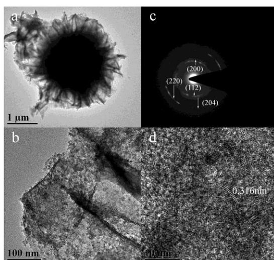
Fig.3 TEM images (a) and (b) of the as-synthesized CMTS particles dispersed in ethanol with SAED pattern (c) and HRTEM image (d)
