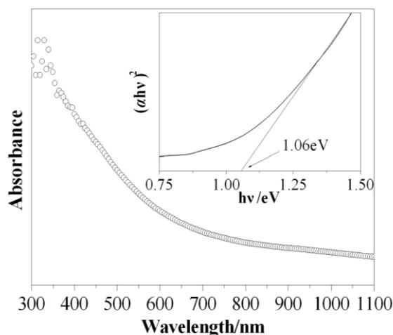
Fig.5 UV-vis-NIR absorption spectrum of the CMTS particles
