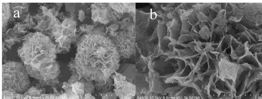
Fig.2 SEM images of the as-synthesized CMTS particles with low (a) and high (b) magnifications
