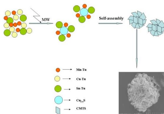
Fig.4 The growth mechanism of the as-synthesized CMTS particles
