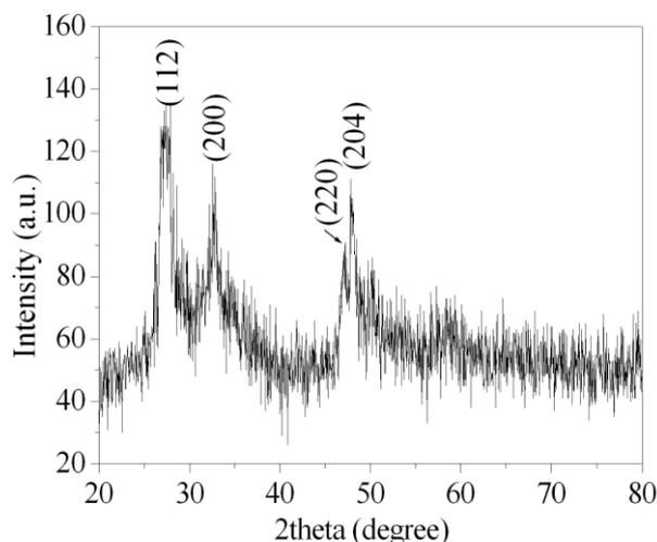
*Fig.1 X-ray diffraction pattern of the as-synthesized CMTS particles*
