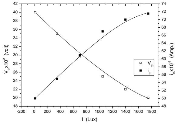
Fig. 9: Dependence of  $\ell_{th}$  and  $V_{th}$  on the illumination of  $TlBiS_2$  compound.
