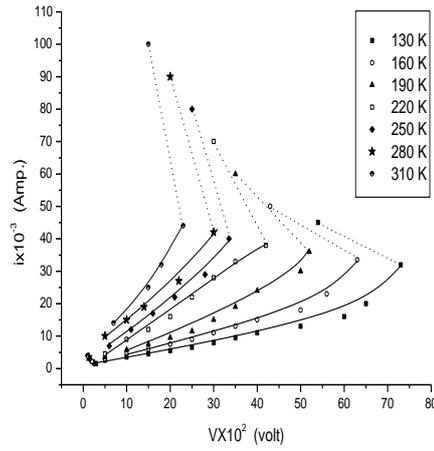
Fig. 2: CVC at different values of temperature for a TlBiS<sub>2</sub> single crystal
