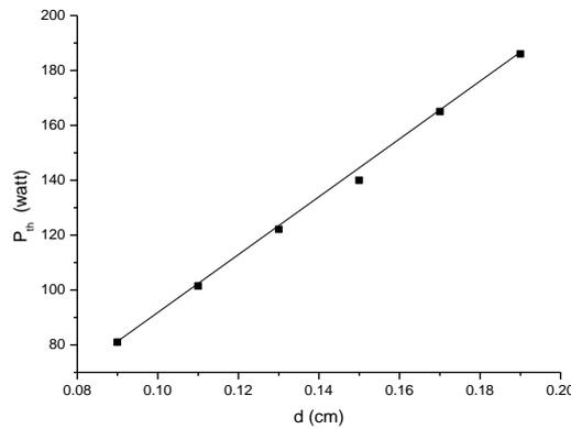
Fig. 15: Variation of threshold power  $P_{th}$  with the thickness of the TlBiS<sub>2</sub> single crystal
