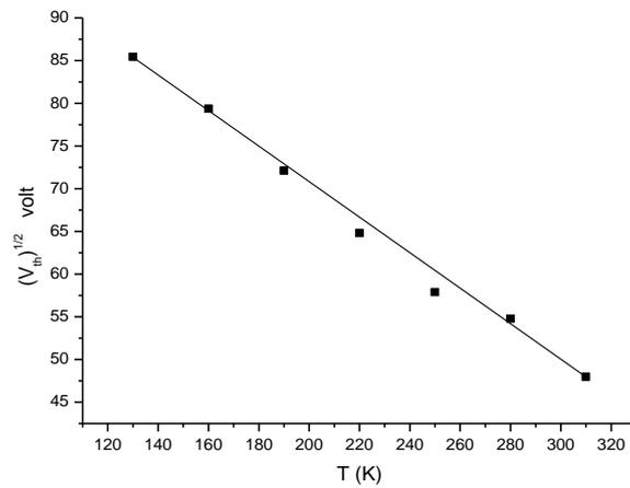
Fig. 5: Temperature dependence of  $\sqrt{V_{th}}$  for the  $TlBiS_2$  compound
