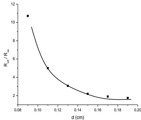
Fig. 16: Effect of thickness of the active region of TlBiS<sub>2</sub> sample on the ratio  $R_{OFF}/R_{ON}$
