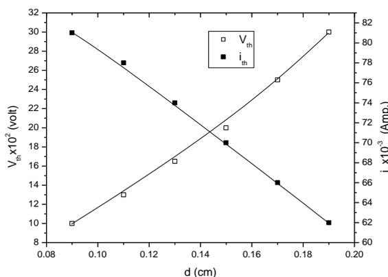
Fig.13: Variation of  $V_{th}$  and  $I_{th}$  with the thickness of TlBiS<sub>2</sub> sample
