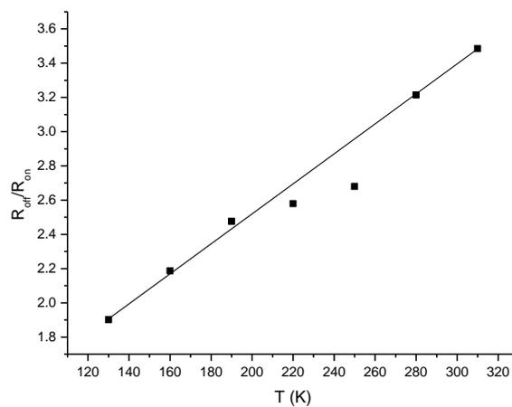
Fig.7: Ambient temperature effect on the sample resistance ratio ( $R_{OFF}/R_{ON}$ ) of  $TlBiS_2$
