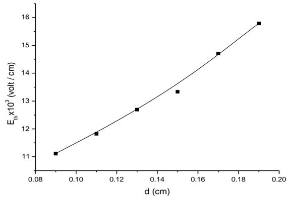
Fig. 14: The dependence of threshold field  $E_{th}$  on the thickness of the TlBiS<sub>2</sub> sample
