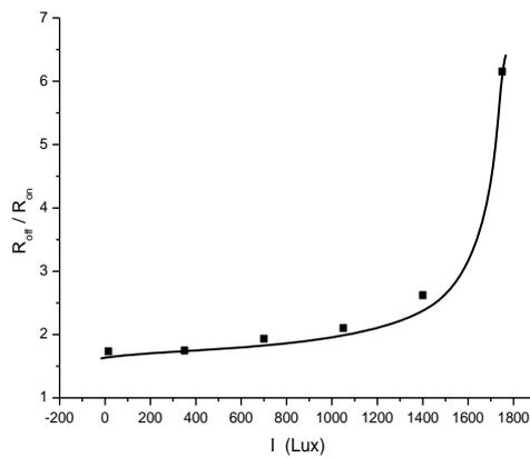
Fig. 11: Effect of illumination intensity on the ratio  $R_{OFF}/R_{ON}$ .
