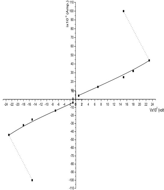
Fig. 1: Symmetrical behavior of the CVC of TlBiS<sub>2</sub> relative to the polarity
