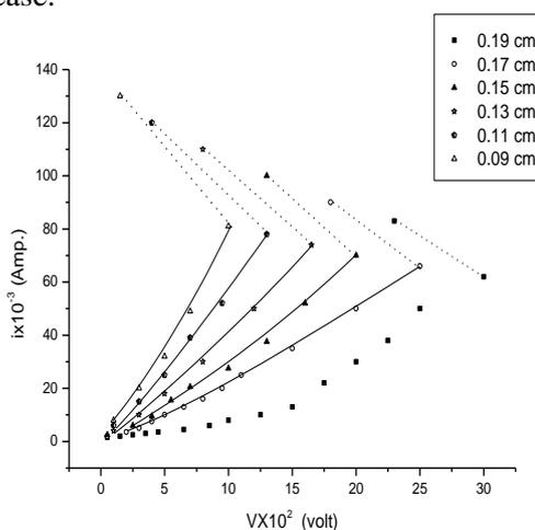
Fig. 12: CVC for TlBiS<sub>2</sub> compound with various sample thickness
