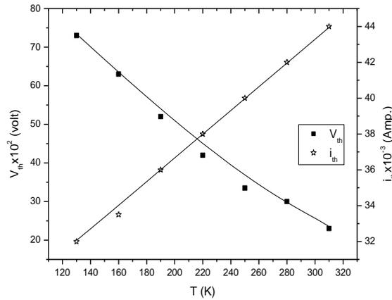
Fig. 3: Effect of surrounding temperature on the threshold current and voltage for TlBiS<sub>2</sub> single crystal
