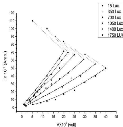
Fig.8: Influence of light intensity on the  $I-V$  characteristics of  $TlBiS_2$  single crystals
