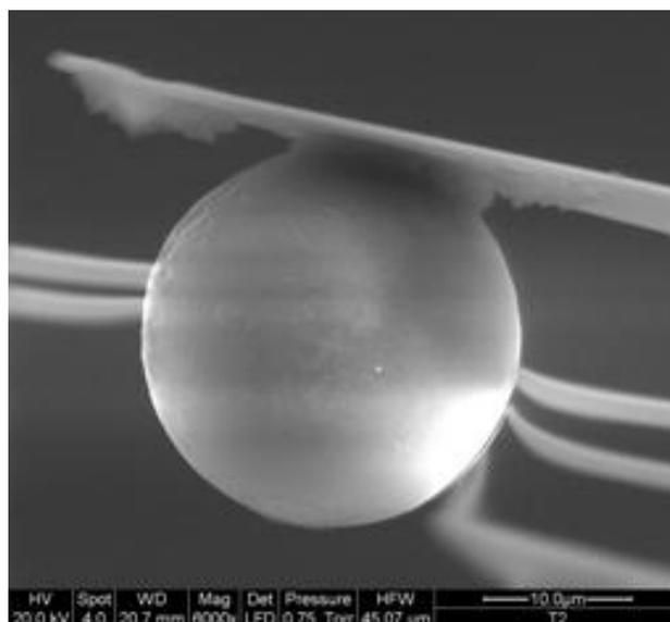
Fig. 1b. SEM pictures of attached spheres with a  $25\ \mu\text{m}$  diameter.
