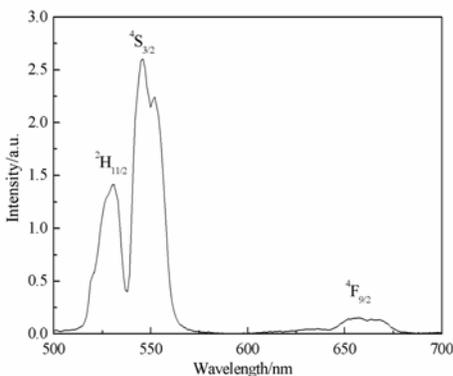
Fig. 2. Upconversion spectrum of 1.0wt% Er<sup>3+</sup>-doped TeO<sub>2</sub>-WO<sub>3</sub> glass.
