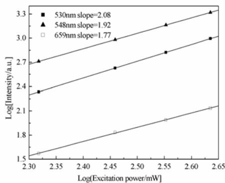
Fig. 3. Dependence of the integrated intensity of upconversion emission on excitation power.
