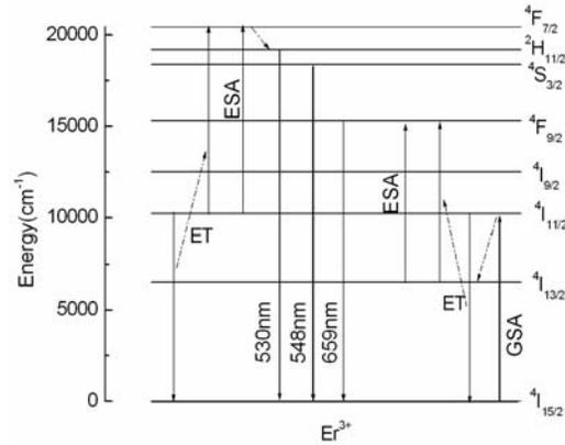
Fig. 4. Energy level diagram of  $\text{Er}^{3+}$  ions and upconversion mechanism in  $\text{Er}^{3+}$ -doped  $\text{TeO}_2\text{-WO}_3$  glass.
