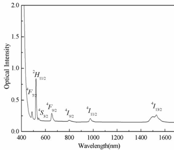
Fig. 1. Absorption spectrum of 1.0wt% Er<sup>3+</sup>-doped TeO<sub>2</sub>-WO<sub>3</sub> glass.
