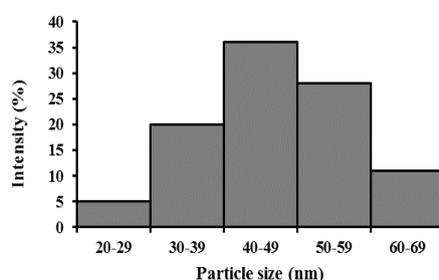
Fig. 1. The particle size distribution of TiO<sub>2</sub> nanoparticles.
