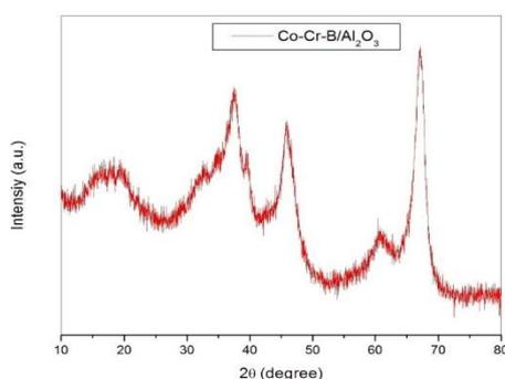
Fig. 7. XRD patterns of  $\text{Co-Cr-B}/\text{Al}_2\text{O}_3$  catalyst.
