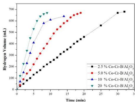
Fig. 4. Hydrogen generation rate of different metal/Al<sub>2</sub>O<sub>3</sub> ratios (reaction condition: concentration of NaOH: 5 wt%; amount of catalyst: 100 mg; concentration of NaBH<sub>4</sub>: 2.5 wt%; temperature: 30 °C).
