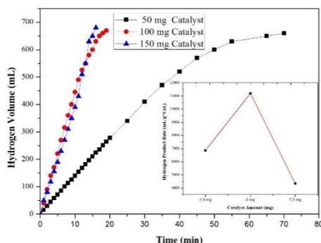
Fig. 3. Hydrogen generation rate of different amount of catalyst (reaction condition: concentration of NaOH: 5 wt%; concentration of NaBH<sub>4</sub>: 2.5 wt%; temperature: 30 °C).
