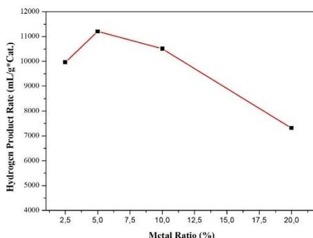
Fig. 5. The maximum value of hydrogen generation of different molar ratios of Co-Cr-B/Al<sub>2</sub>O<sub>3</sub> at 30 °C.
