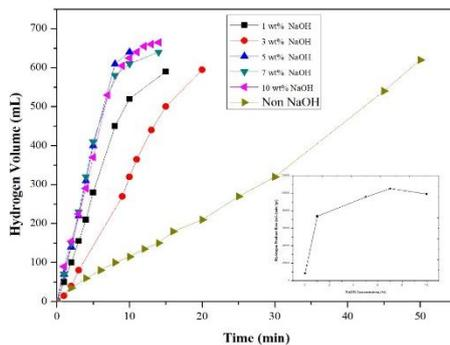
Fig. 1. Hydrogen generation rate of different NaOH concentrations (reaction condition: concentration of  $\text{NaBH}_4$ : 2.5 wt%; amount of catalyst: 100 mg; temperature:  $30^\circ\text{C}$ ).
