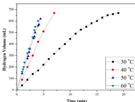
Fig. 6a. Hydrogen generation rate at different temperatures (reaction condition: concentration of NaOH: 5 wt%; amount of catalyst: 100 mg; concentration of NaBH<sub>4</sub>: 2.5 wt%; temperature: 30 °C).
