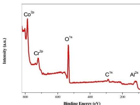
Fig. 8. XPS spectra for  $\text{Co-Cr-B}/\text{Al}_2\text{O}_3$  catalyst.
