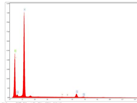
Fig. 9. The EDX spectra of Co-Cr-B /Al<sub>2</sub>O<sub>3</sub> catalyst.
