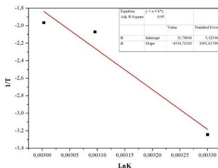
Fig. 6b. The Arrhenius plot for the hydrolysis of  $\text{NaBH}_4$  in the presence of  $\text{Co-Cr-B}/\text{Al}_2\text{O}_3$ .
