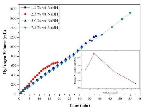
Fig. 2. Hydrogen generation rate of different  $\text{NaBH}_4$  concentrations (reaction condition: concentration of NaOH: 5 wt%; amount of catalyst: 100 mg; temperature:  $30^\circ\text{C}$ ).
