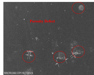
Fig. 2.3.3.3 Sem Analysis of Resin cast with 20 microns zoom
