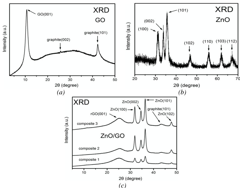
Fig. 1. XRD spectra of a) GO, b) ZnO and c) ZnO/GO composites.
