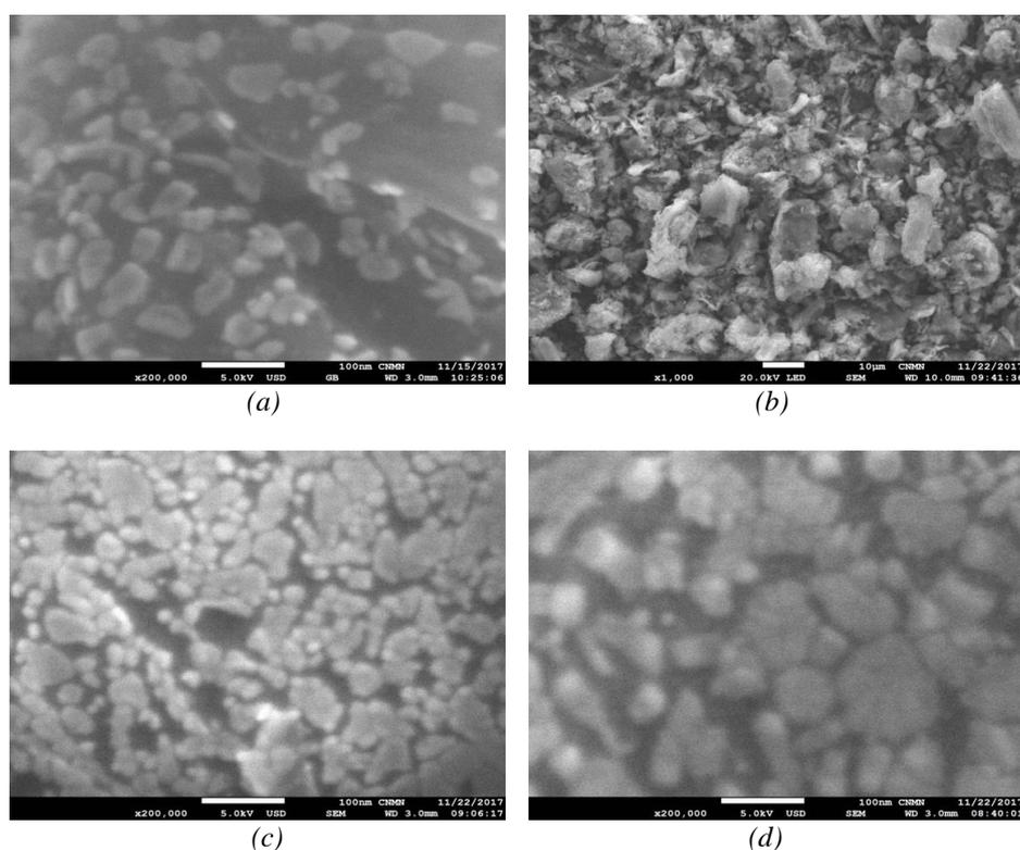
Fig. 3. SEM micrography of a) ZnO/GO composite 1, b)–c) ZnO/GO composite 2, and d) ZnO/GO composite 3.
