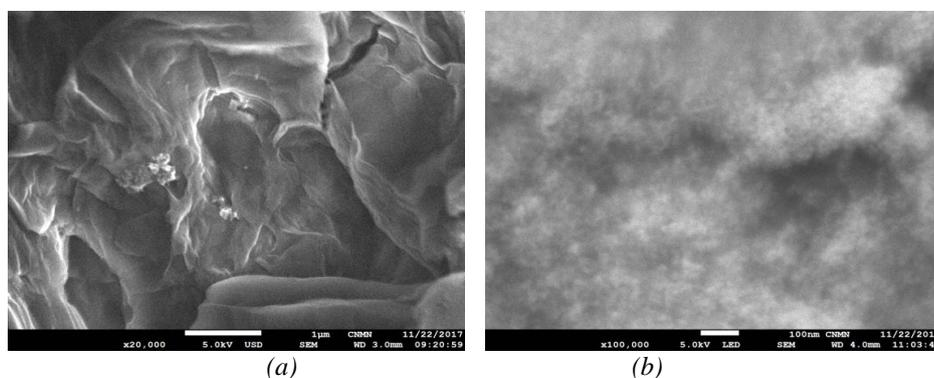
Fig. 2. SEM micrography of a) GO and b) ZnO.
