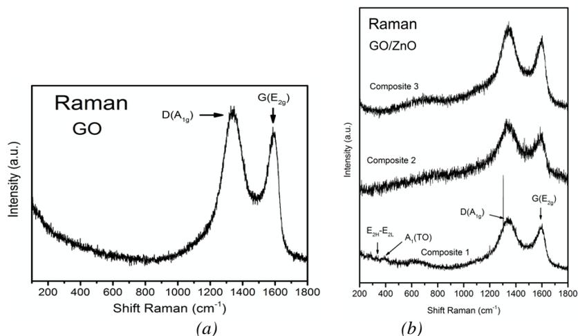
Fig. 4. Raman spectra of a) GO and b) ZnO/GO composites.
