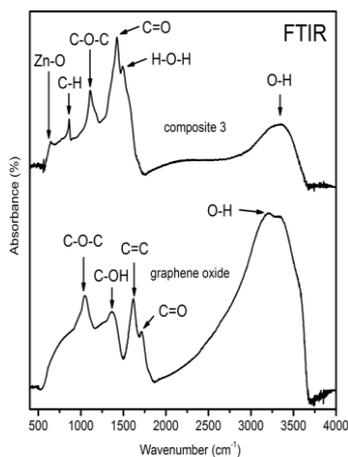
Fig. 5. FTIR spectra of GO and ZnO/GO composite 3.
