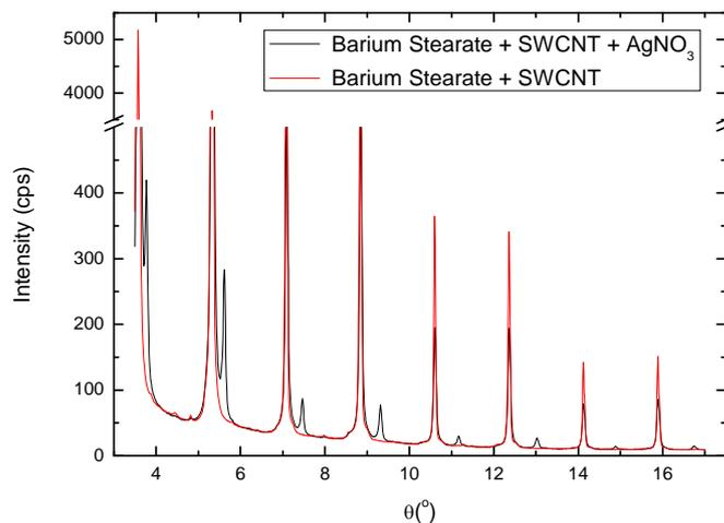
Fig. 4 The X-ray diffraction pattern of the multilayers with carbon nanotubes and without  $\text{AgNO}_3$  and multilayers with  $\text{AgNO}_3$  layers
