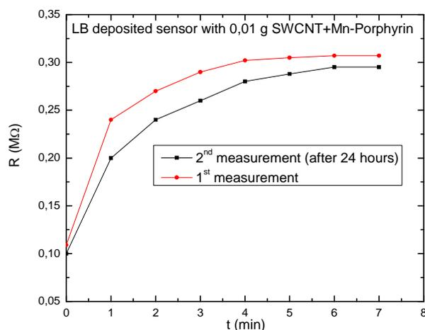
Fig. 3 The effect of UV radiation of the sensor based on nanotubes and Mn-porphyrin.
