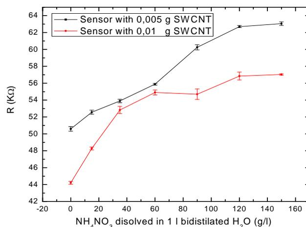
Fig.2 The plot of the resistance of the sensor immersed in the test solution as a function of ammonium nitrate concentration for two sensing bodies with different concentration of carbon nanotubes.
