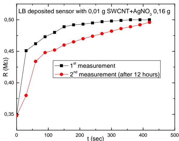
Fig.5 The effect of UV radiation of the sensor based on nanotubes and  $\text{AgNO}_3$
