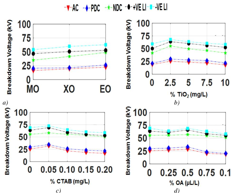
Fig. 10 Break down voltage (BDV) for a) MO, XO and EO; b) NO; c) CNO; ONO.
