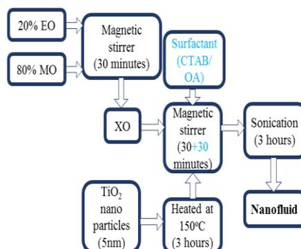
Fig. 2. Procedure for the preparation of NO.
