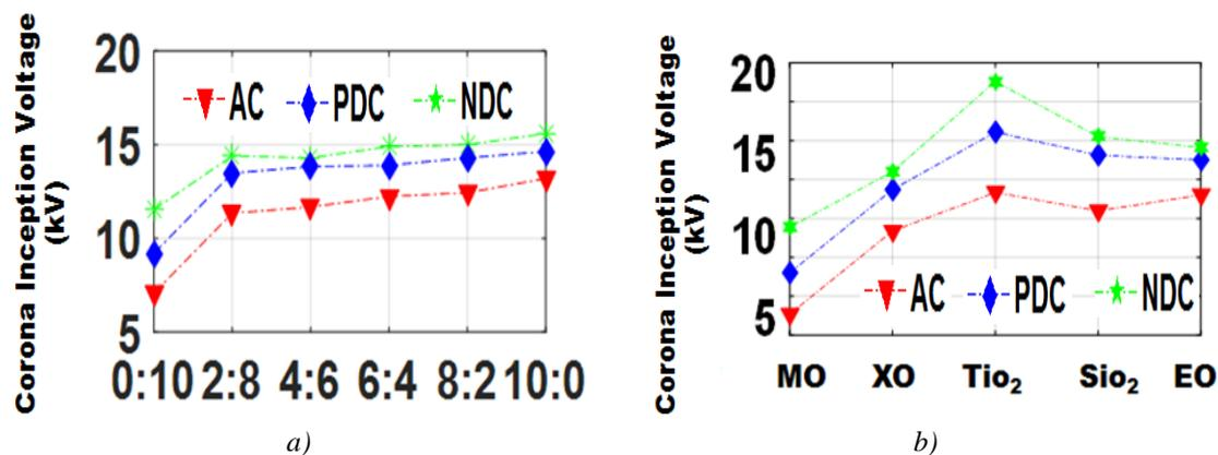
Fig. 6. Corona Inception Voltage under different voltages for different proportions of a) MO and EO; b) MO, XO, XO+ $TiO_2$ , XO+ $SiO_2$ , EO.
