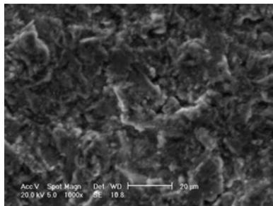
*Fig. 11 Biological hydroxyapatite layer deposited after 15 days of immersion in 1.5 SBF on P3 sample surface (SEM image).*
