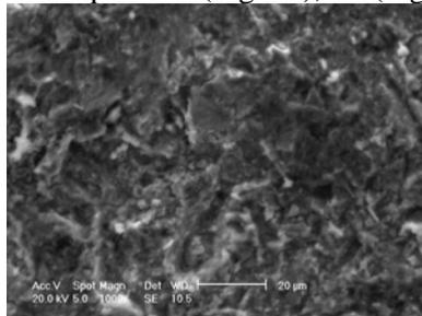
*Fig. 12 Biological hydroxyapatite layer deposited after 21 days of immersion in 1.5 SBF on P1 sample surface (SEM image).*
