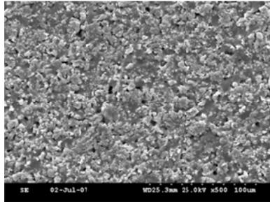
Fig. 17 Hydroxyapatite deposited on P1 sample (SEM image x 500).
