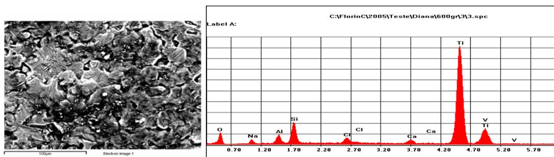
Fig. 5 SEM image and X-ray diffraction of the surface of P3 sample sandblasted with  $\text{SiO}_2$ , attacked by 10M NaOH solution for 24 h at  $60^\circ\text{C}$  and subjected to heat treatment for 1 hour at  $600^\circ\text{C}$ .
