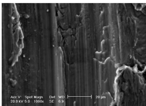
*Fig. 1. SEM image of the surface of P1 titanium sample obtained by sandblasting*
