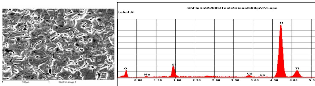
Fig. 3. SEM image and X-ray diffraction of the surface of P1 sample sandblasted with  $\text{SiO}_2$ , attacked by 10M NaOH solution for 24 h at  $60^\circ\text{C}$  and subjected to heat treatment for 1 hour at  $600^\circ\text{C}$ .
