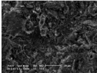
*Fig. 10 Biological hydroxyapatite layer deposited after 15 days of immersion in 1.5 SBF on P2 sample surface (SEM image).*
