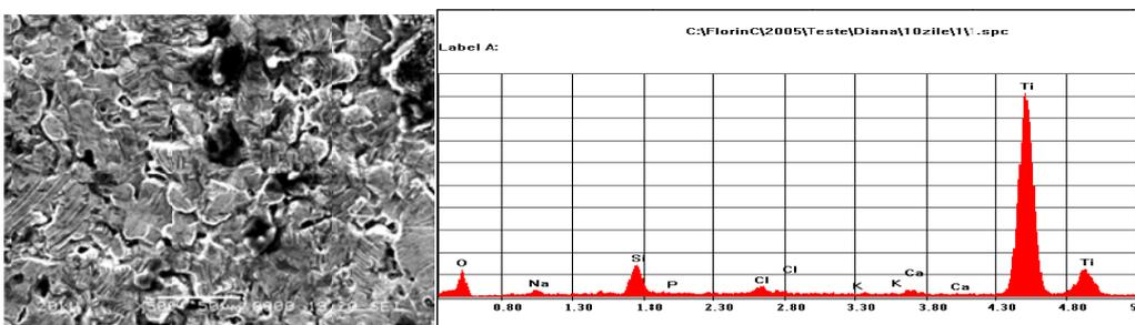
*Fig. 22 SEM image of P3 sample surface, sandblasted, after ten days of immersion in SBF and 1.5 SBF and the composition of the superficial layer by EDX image*
