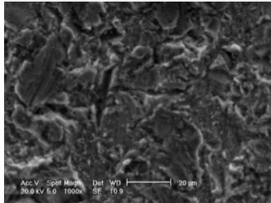
*Fig. 14 Biological hydroxyapatite layer deposited after 21 days of immersion in 1.5 SBF on P3 sample surface (SEM image).*
