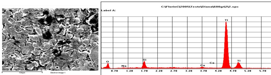
Fig. 4. SEM image and X-ray diffraction of the surface of P2 sample sandblasted with  $\text{SiO}_2$ , attacked by 10M NaOH solution for 24 h at  $60^\circ\text{C}$  and subjected to heat treatment for 1 hour at  $600^\circ\text{C}$ .
