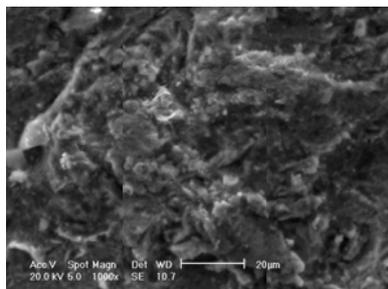
*Fig. 9 Biological hydroxyapatite layer deposited after 15 days of immersion in 1.5 SBF on P1 sample surface (SEM image).*
