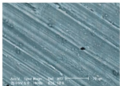
*Fig. 2. SEM image of the surface of P2 titanium sample abraded by diamond files.*
