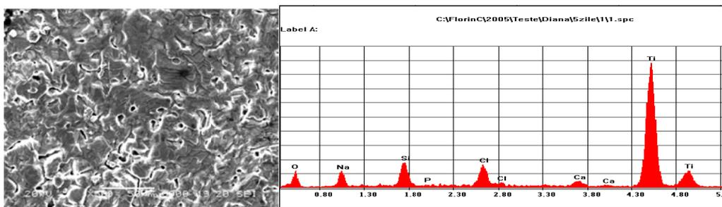
*Fig. 21 SEM image of P3 sample surface, sandblasted, after five days of immersion in SBF and 1.5 SBF and the composition of the superficial layer by EDX image*
