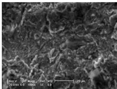
*Fig. 13 Biological hydroxyapatite layer deposited after 21 days of immersion in 1.5 SBF on P2 sample surface (SEM image).*
