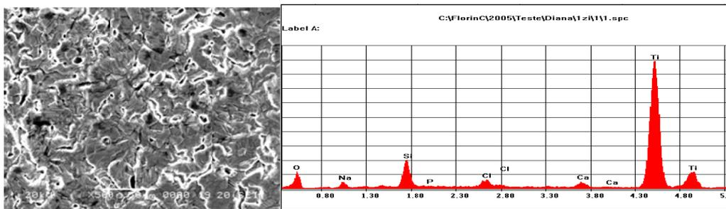
*Fig. 20 SEM image of P3 sample surface, sandblasted, after one day of immersion in SBF and the composition of the superficial layer by EDX image*
