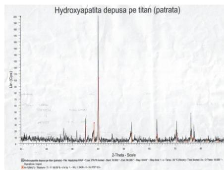
*Fig. 16 Biological hydroxyapatite layer deposited after 15 days of immersion in 1.5 SBF on P2 sample surface (diffractogram).*
