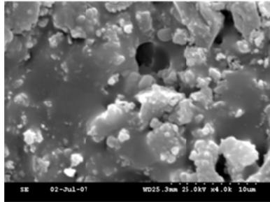
Fig. 18 Hydroxyapatite deposited on P1 sample (SEM image x 4000).
