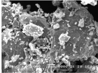
*Fig. 6 SEM image of P1 titanium sample after 3 days of immersion in SBF (one day in SBF and two days in 1.5 SBF).*
