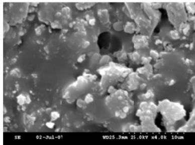
*Fig. 8 SEM image of P1 titanium sample after 3 days of immersion in SBF (one day in SBF and two days in 1.5 SBF).*
