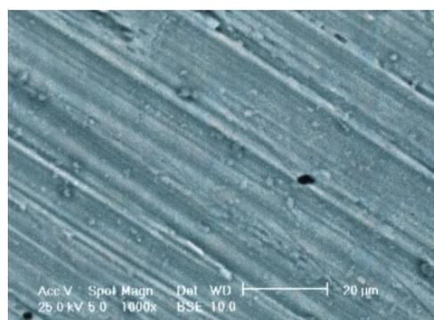
*Fig. 2. SEM image of the surface of P2 titanium sample abraded by diamond files.*
