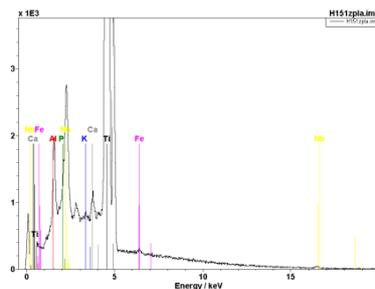
Fig. 19 Hydroxyapatite deposited on P1 sample (X-ray diffraction). The high-intensity black peaks are assigned to hydroxyapatite and the red ones are assigned to the titanium support.
