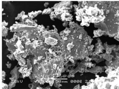
*Fig. 7 SEM image of P2 titanium sample after 3 days of immersion in SBF (one day in SBF and two days in 1.5 SBF).*
