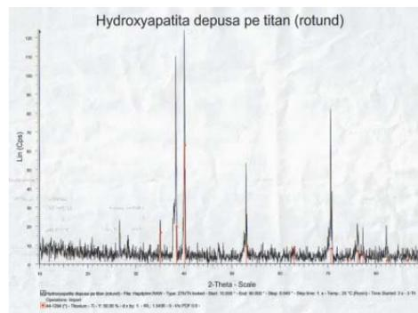
*Fig. 15 Biological hydroxyapatite layer deposited after 15 days of immersion in 1.5 SBF on P1 sample surface (diffractogram).*
