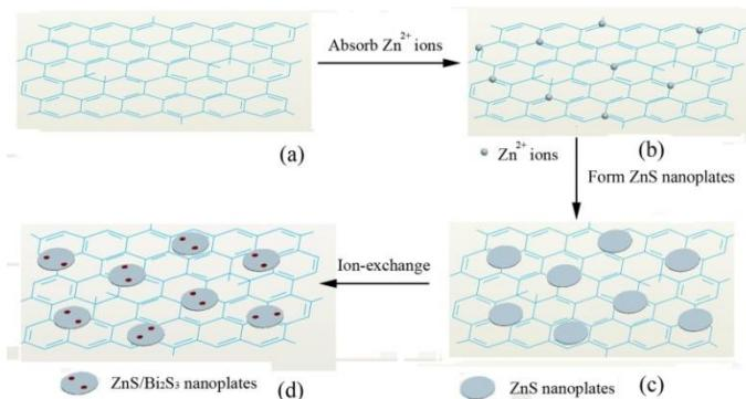
Scheme 1. Proposed scheme of the fabricated processes of G-ZnS/Bi<sub>2</sub>S<sub>3</sub> NP.
