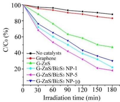
Fig. 7. Photocatalytic degradation efficiency of MO with different catalysts under visible light.
