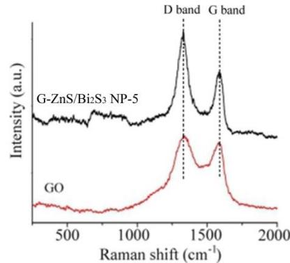
Fig. 3. Raman spectra of GO and G-ZnS/Bi<sub>2</sub>S<sub>3</sub> NP-5 nanocomposites.
