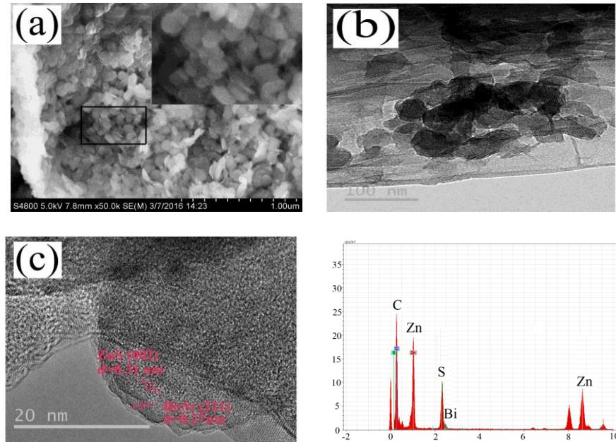
Fig. 5.(a) SEM, (b)TEM. (c)HRTEM, (d)EDX of G-ZnS/Bi<sub>2</sub>S<sub>3</sub> NP-5 nanocomposites
