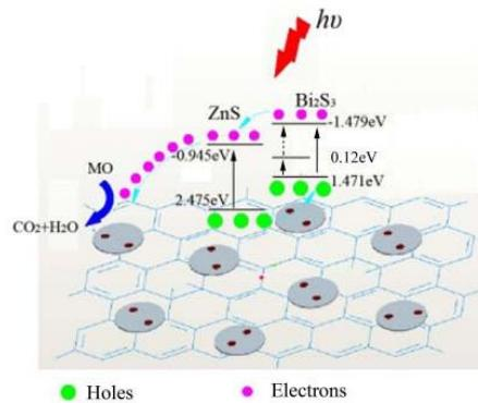
Scheme 2. Schematic illustration for the charge transfer and separation in the G-ZnS/Bi<sub>2</sub>S<sub>3</sub> NP system.
