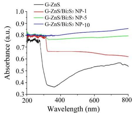
Fig. 4. The UV-vis diffuse reflectance spectra of nanocomposite
