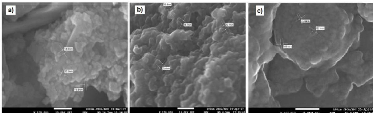
Fig. 2. SEM images of PP/PbS(a) ,PP/CdS (b) and PP+PbS/CdS (c) nanocomposites.
