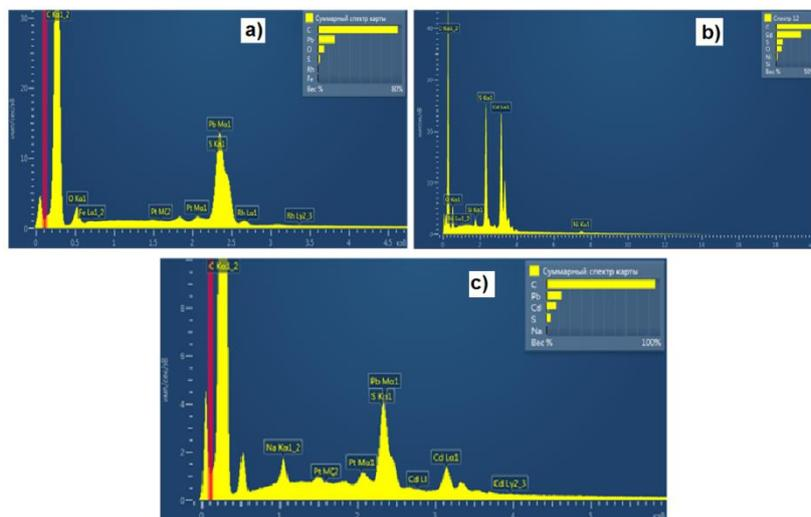
Fig. 3. EDS spectra of PP/PbS(a), PP/CdS (b) and PP+PbS/CdS (c) nanocomposite
