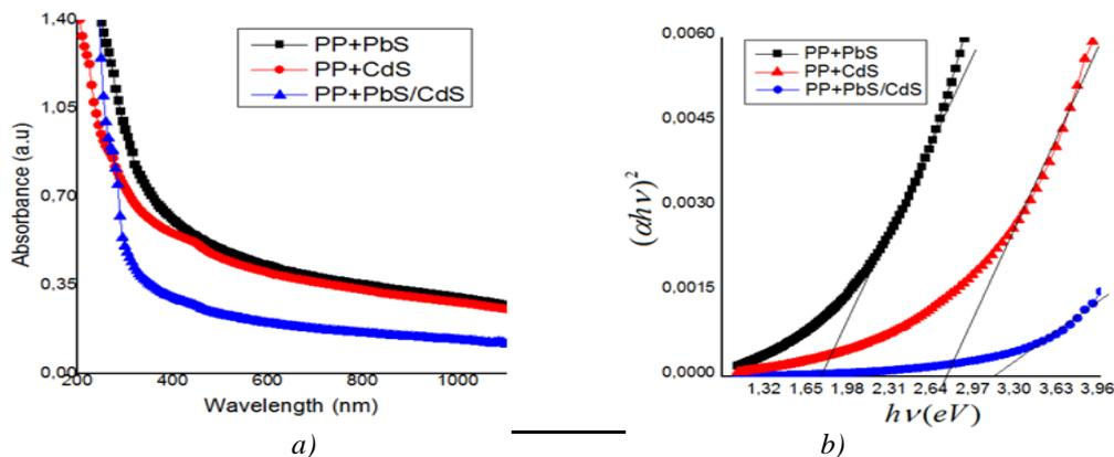
Fig. 1. UV absorptions spectra (a) and band gap calculation (b) for PP/PbS ,PP/CdS and PP+PbS/CdS nanocomposites
