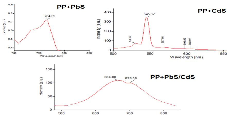
Fig. 4. Photoluminescence spectrum of PP/PbS, PP/CdS and PP+PbS/CdS Nanocomposites
