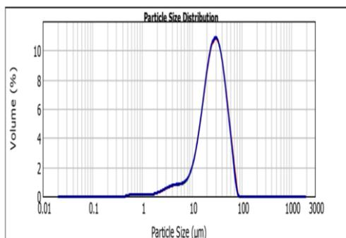
Fig. 4. Particle size distributions of lead selenide quantum dots.
