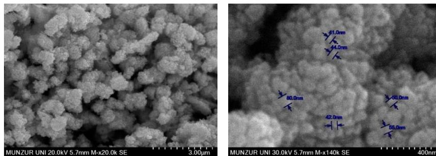
Fig. 7. SEM images of chitosan-coated PbSe quantum dots.
