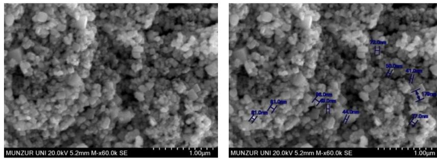
Fig. 6. SEM images of PbSe quantum dots spots.
