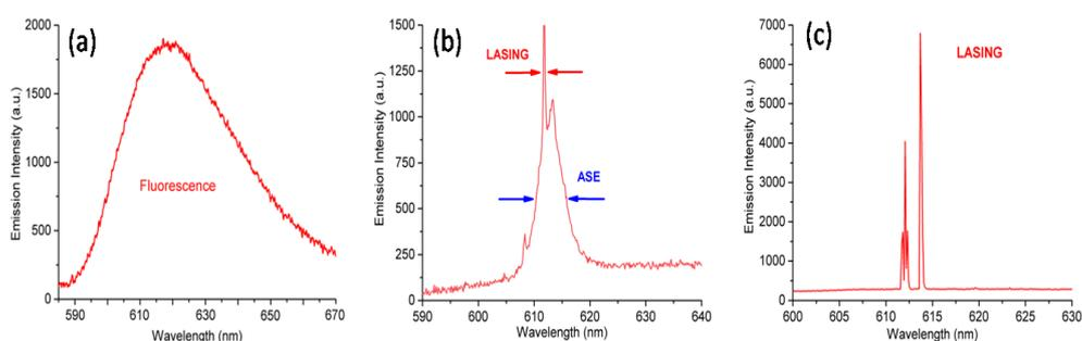
*Fig. 4. Emission spectra from a wedge sample cell under micro-array pumping conditions for increasing input energies. (a) Regular fluorescence spectrum obtained for under-threshold pumping situation. (b) Spectrum acquired for near the threshold energy conditions (one can notice both ASE and emerging lasing peaks). (c) Spectrum for lasing in beyond energy threshold situation*
