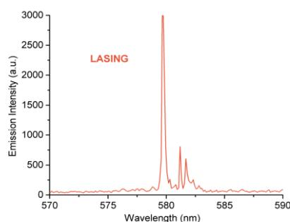
*Fig. 3. Random lasing spectrum from the capillary sample (each lasing mode has a FWHM of ca. 0.5 nm)*
