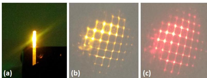
*Fig. 2. (a) Picture of the lasing action from a cylindrical capillary sample. (b-c) Picture showing the On-Screen pattern of random laser micro-array emitters obtained by optically exciting wedge cell samples with the special micro-lenses system (Yellow (b) and Red (c) emissions are shown respectively).*
