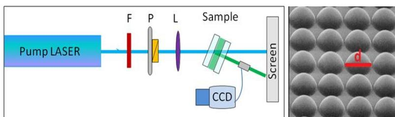
*Fig. 1. (left) Experimental set-up for our study (F – an energy attenuator filter; P – optical polarizer; L – spherical lens; CCD – fiber Charged Coupled Device multichannel spectrometer). (right) Array of micro-lenses (from Thorlabs) used for creating a microstructured emission (d equals ca. 150 microns is the diameter of each plano-convex spherical micro-lens).*
