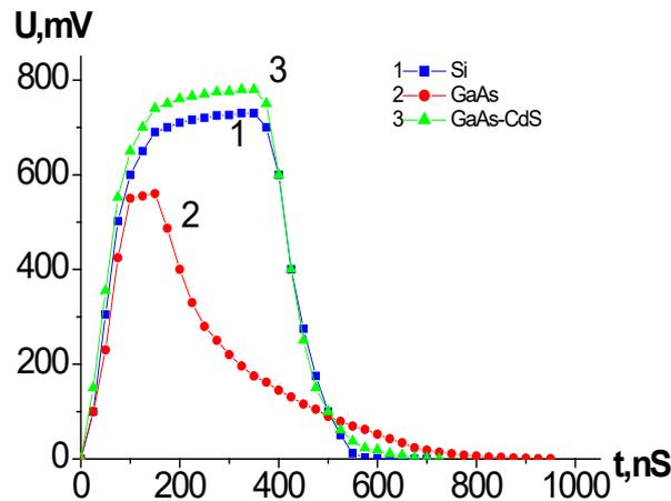
Fig. 5. Pulse shape generated on photodiodes: Au-nSi-Au; Au-vGaAs-Au; Au-vGaAs:O-nCdS-nInP-Au.
