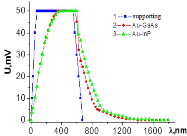
Fig. 4. The shape of the reference pulse and photocurrent pulses when illuminating the Au-nInP-nCdS-vGaAs:O-Au photodetector with a rectangular light pulse from different surfaces.
