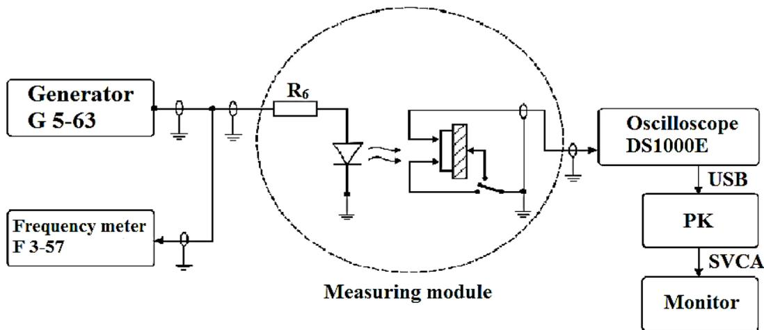
Fig. 1. Electrical circuit for measuring the time characteristics of photodiode structures.
