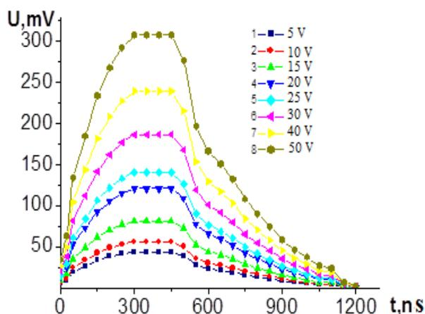
Fig. 6. Pulse shape generated on the Au-nInP-nCdS-vGaAs:O-Au photodiode from a rectangular light pulse with a wavelength of 1300 ns at different blocking voltages.
