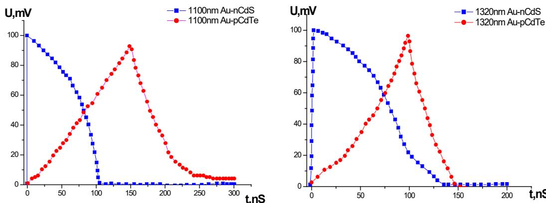
Fig. 3. The shape of the photocurrent pulses when illuminating an Au-nCdS-nSi-pCdTe-Au photodiode with a rectangular light pulse from different surfaces. a) When illuminating a photodiode with a light-emitting diode with a wavelength of  $\lambda=1100$  nm on the surface from the side of Au-nCdS and pCdTe-Au; b) When illuminating a photodiode with a light-emitting diode with a wavelength of  $\lambda=1320$  nm onto the surface from the side of Au-nCdS and pCdTe-Au.
