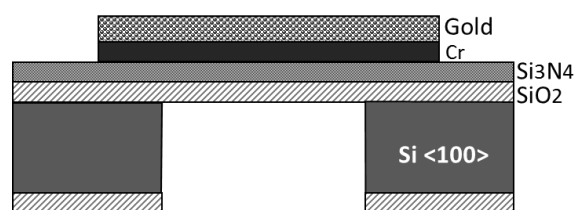
Fig. 1. Cross-section of the final structure (not at scale)
