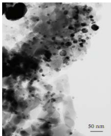
Fig. 4. TEM micrograph of silver nanoparticles loaded on hydroxyapatite.
