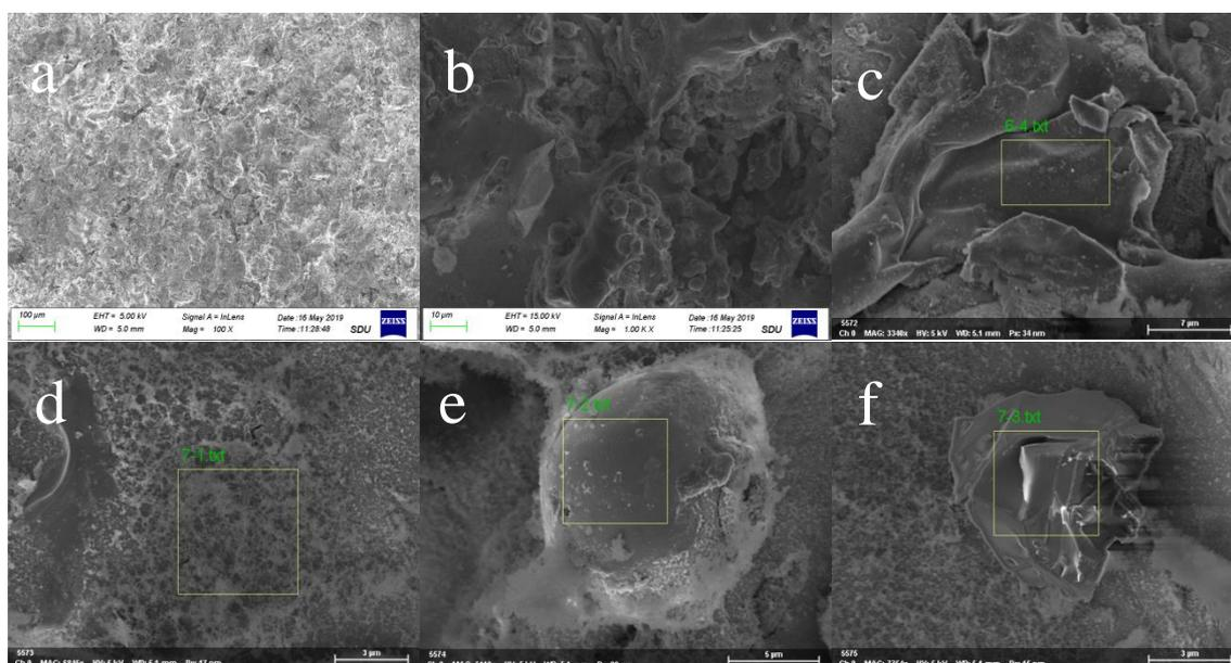
Fig. 5. SEM images of Metco 404NS coating surface morphology and its different areas: (c) smooth surface area, (d) flocculation area, (e) globular region, (f) block area.
