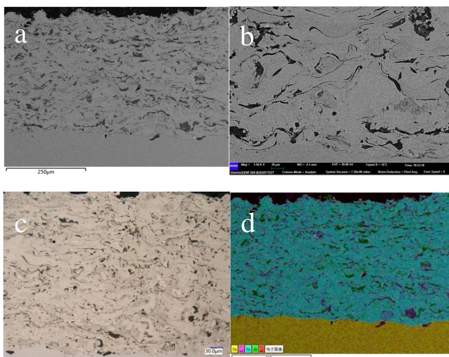
Fig. 8. Cross-section SEM images of Metco 404NS coating.
