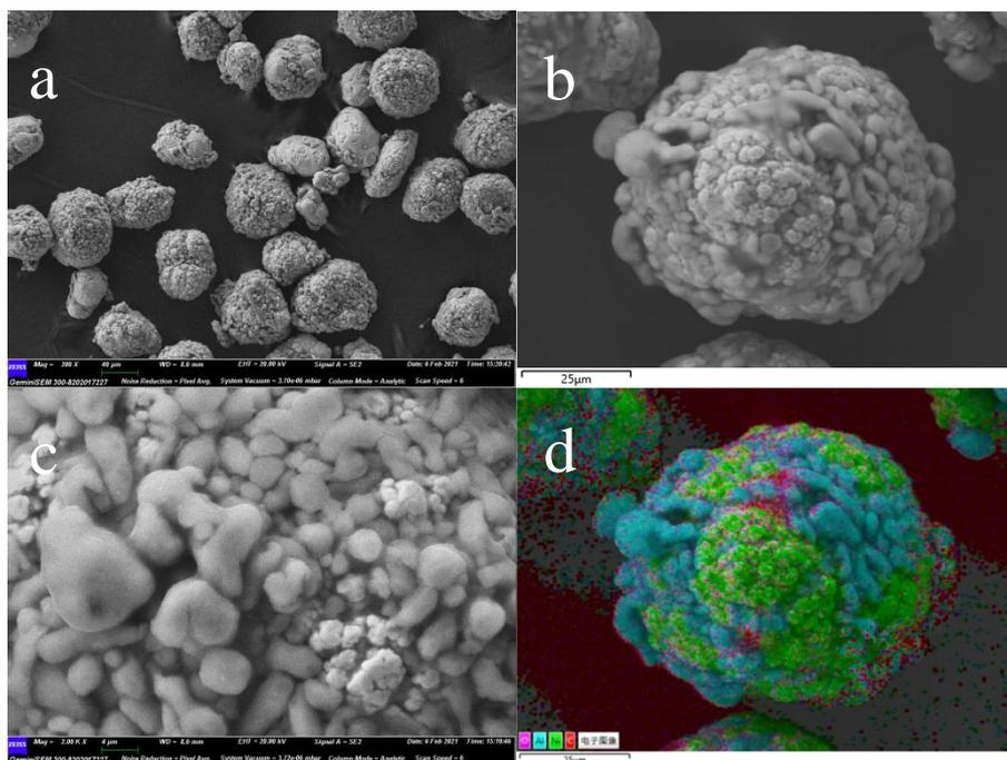
Fig. 2. SEM micrographs of Metco 404NS powder.
