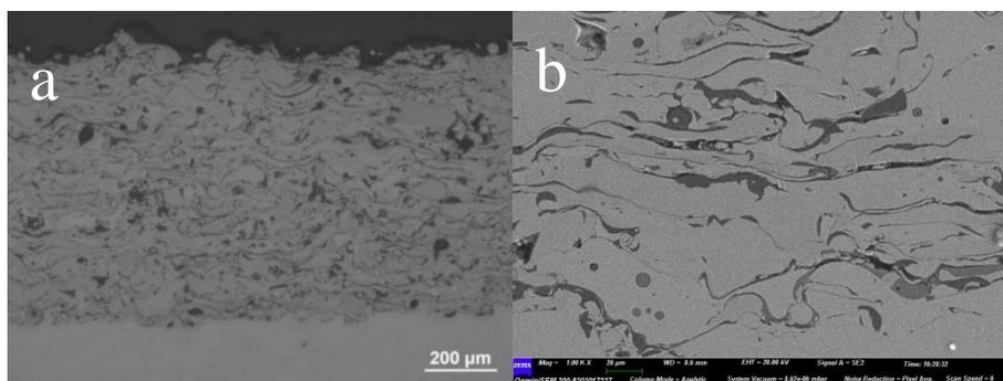
*Fig. 17. Coating section formed by flame spraying Metco 405NS composite wire.*
