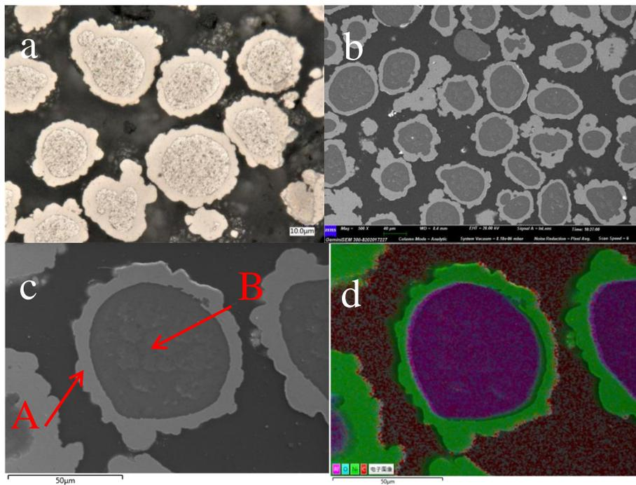
Fig. 3. Cross-section of Metco 404NS powder.
