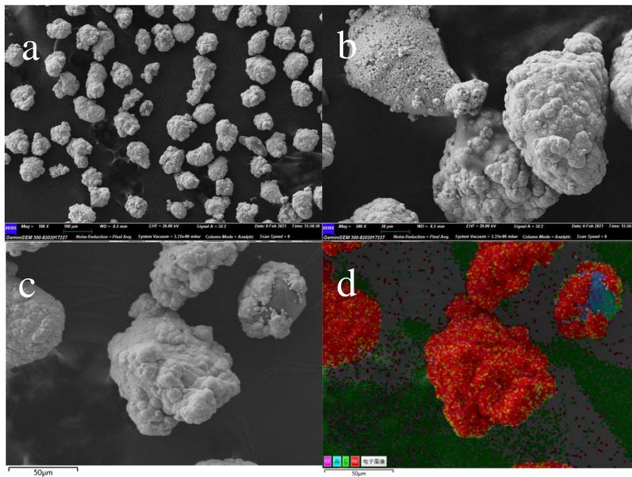
Fig. 1. SEM micrographs of Metco 404NS powder.
