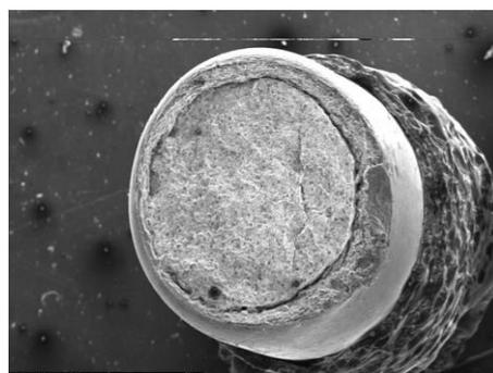
Fig. 15. Section photo of Metco 405NS (80% Nickel / 20% Aluminum) composite wire.
