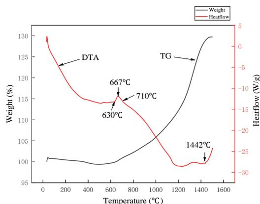
Fig. 11. The TG/DTA curves of the Metco 450NS powders.
