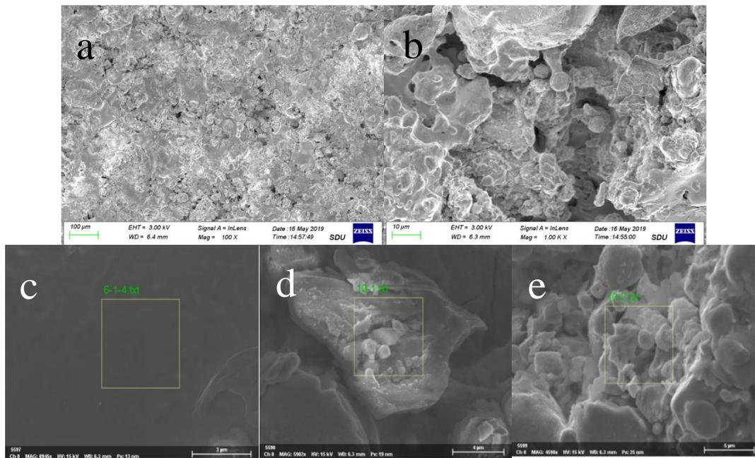
Fig. 7. SEM images of Metco 450S coating surface morphology and its different areas: (c) smooth surface area, (d) block area, (e) unmelted particles.
