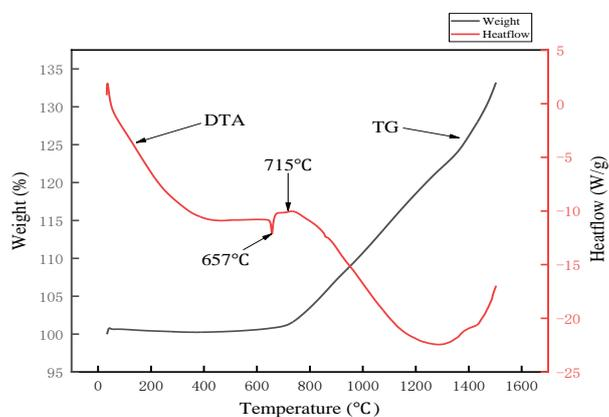
Fig. 10. The TG/DTA curves of the Metco 404NS powders.
