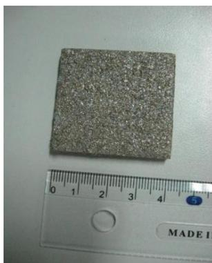
*Fig. 16. Photo of coating surface formed by flame spraying Metco 405NS (80% Nickel / 20% Aluminum) composite wire.*
