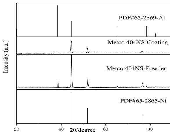
Fig. 12. XRD spectra of Metco 404NS coating and powder.
