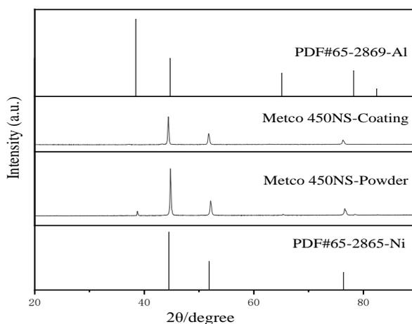
Fig. 13. The XRD spectra of Metco 450NS coating and powder.
