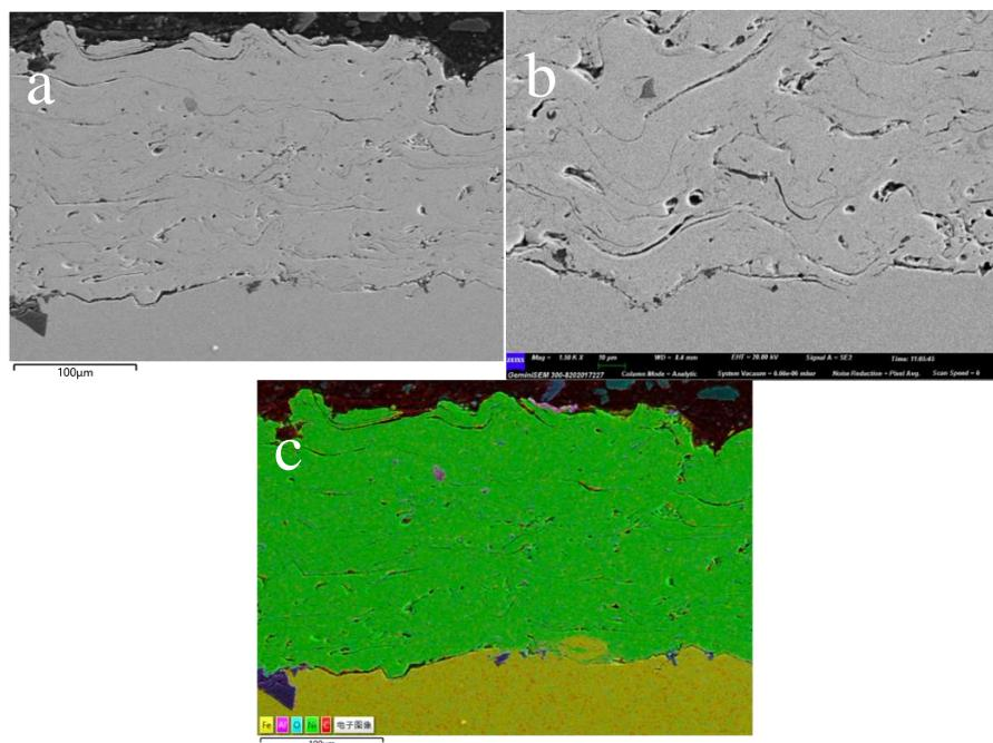
Fig. 9. Cross-section SEM images of Metco 450NS coating.
