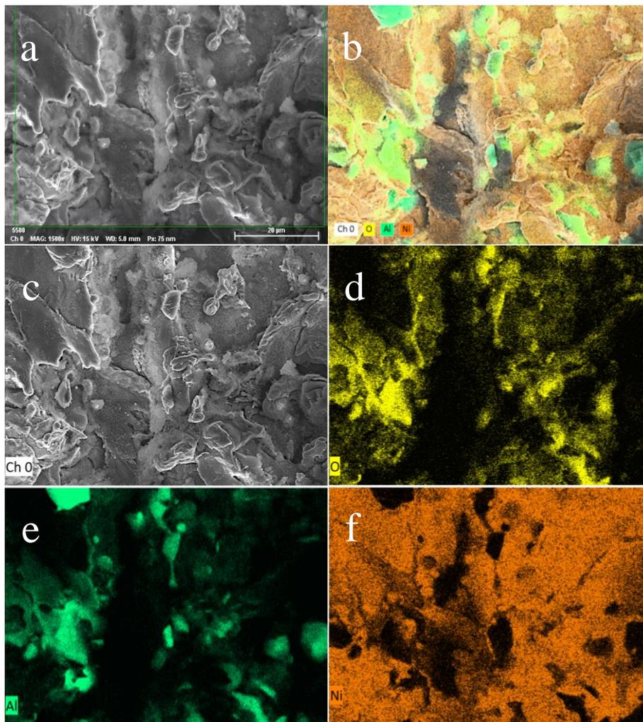
Fig. 6. SEM images of Metco 404NS coating surface morphology and EDS element mapping.
