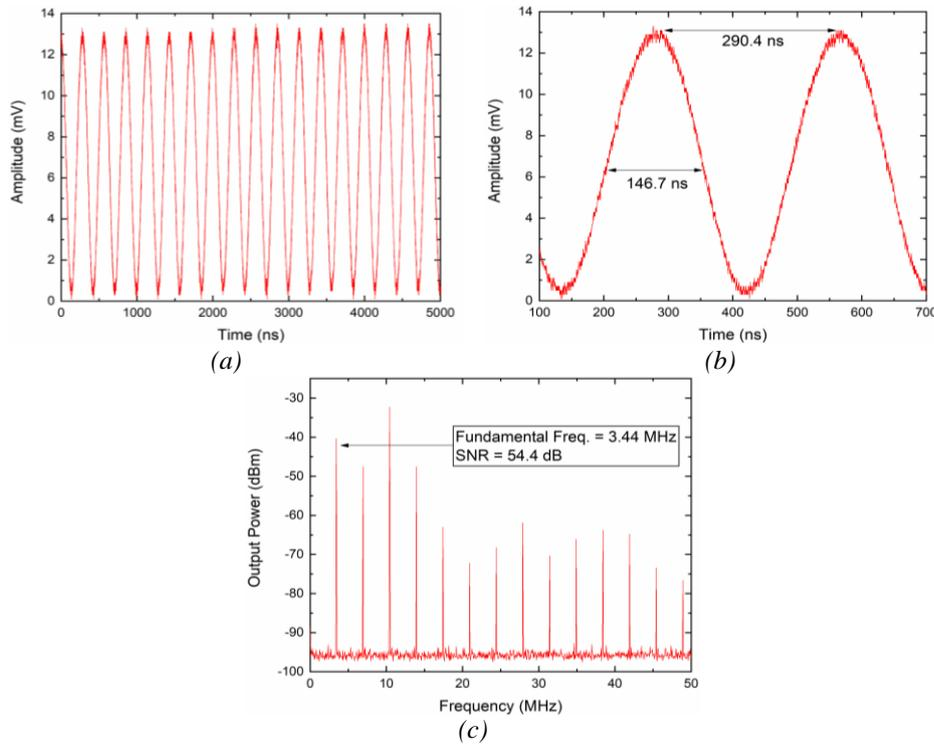
Fig. 3. Temporal performances of the generated SPL; (a) oscilloscope spectrum, (b) two pulses envelopes, and (c) radio frequency spectrum.
