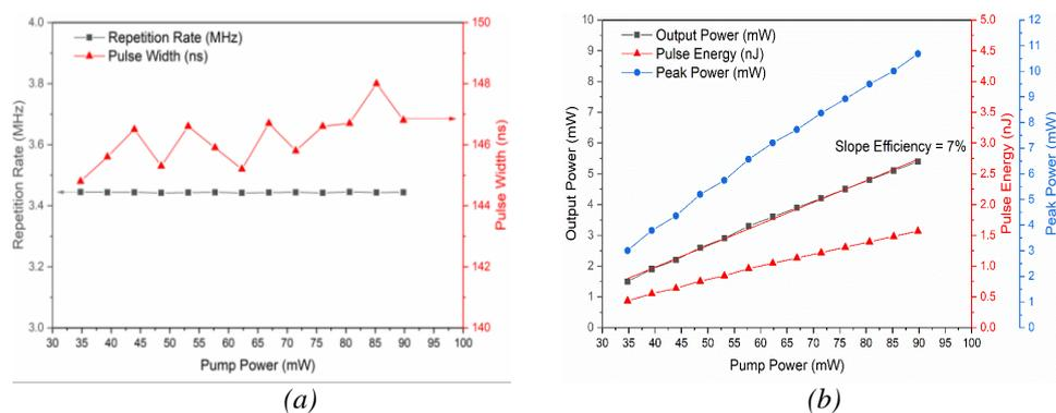
Fig. 4. SPL performances with the variation of pump power; (a) The graph of repetition rate and pulse width as a function of pump power, and (b) the graph of output power, pulse energy, and peak power as a function of pump power.
