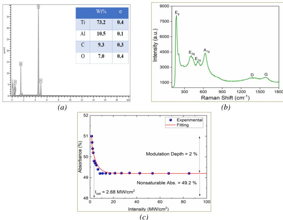
Fig. 1. Characterization of  $\text{Ti}_3\text{AlC}_2$ : (a) EDS spectrum, (b) Raman spectrum, (c) nonlinear absorption profile at 1.55- $\mu\text{m}$  region.
