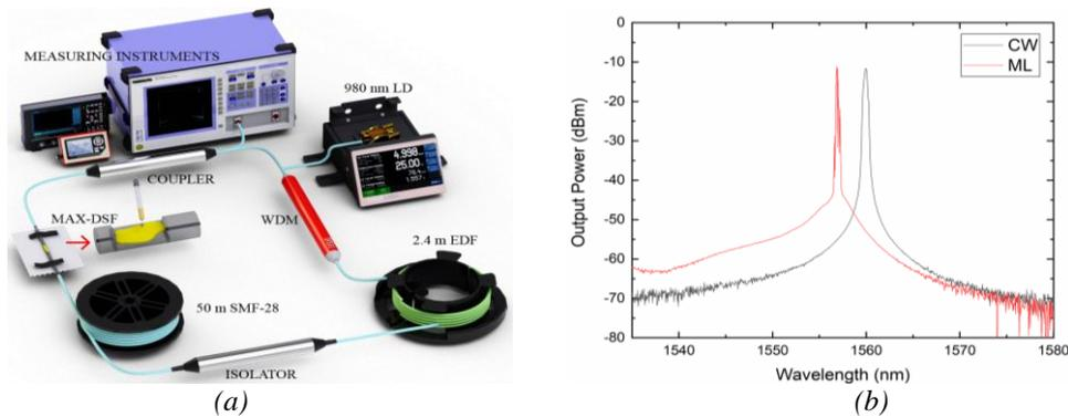
Fig. 2. (a) Experimental configuration for nanosecond pulse generation in an EDFL cavity with a  $\text{Ti}_3\text{AlC}_2$  deposited onto D-shaped fiber as SA. (b) generated optical spectrum at continuous wave and mode-locked operation.
