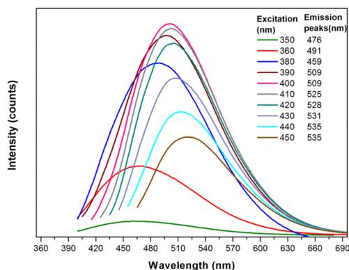
Fig. 7. PL emission spectra recorded for excitation wavelengths from 350 to 450 nm for the prepared C-dots dispersed in acetone
