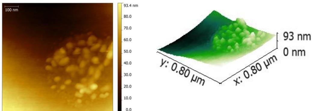
Fig. 5. (a) Recorded AFM image; (b) projected 3D image of the C-Dots
