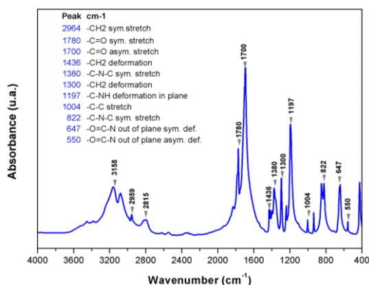
Fig. 2. FT-IR spectrum recorded for the prepared C-Dots including functional groups assignment
