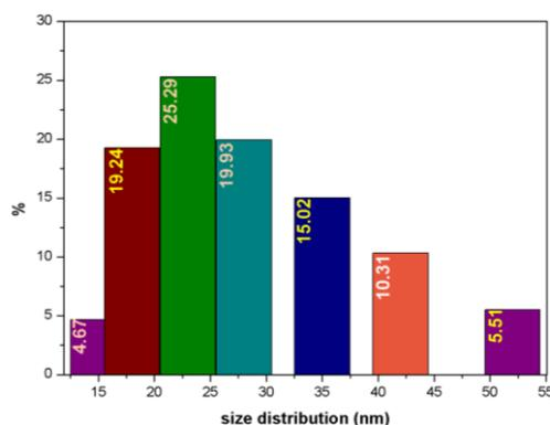
Fig. 4. Size distribution of the prepared C-Dots
