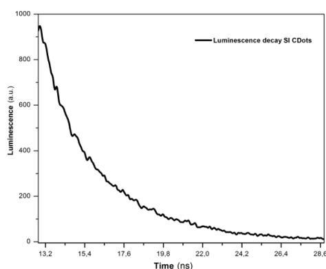
Fig. 8. Luminescence decay recorded for the investigated C-Dots dispersed in acetone
