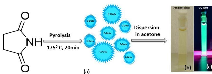
Fig. 1.(a) Schematic illustration of the C-Dots preparation path, (b) C-Dots dispersed in acetone in ambient lighting conditions, (c) under UV-A excitation
