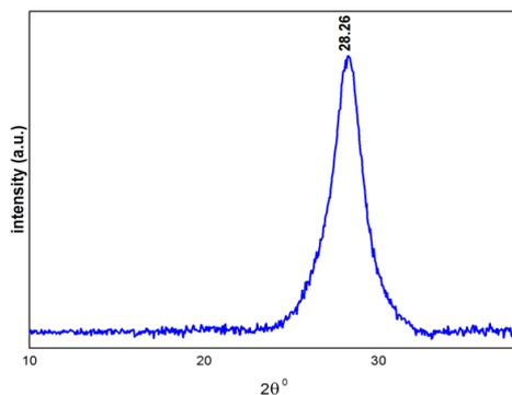
Fig 3. Recorded XRD pattern of the prepared C-Dots
