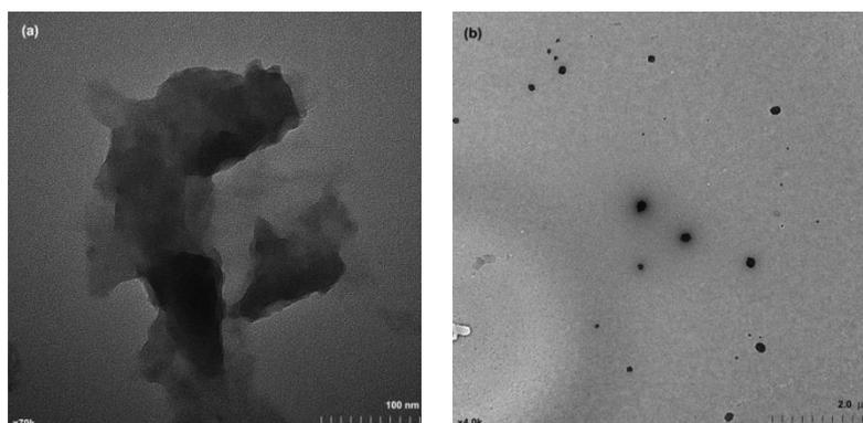
Fig. 6. TEM micrographs recorded for the investigated C-dots
