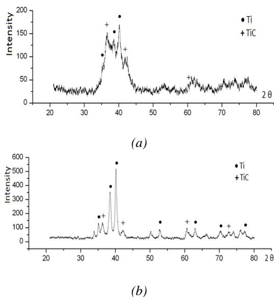
Fig. 7. X-ray diffraction pattern of a sample of the composition Ti + 4 wt. % CNTs after 8 min. MA.
