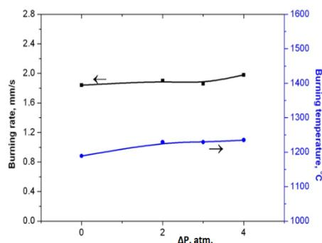
Fig. 10. Dependence of the temperature and combustion rate of the delay composition on the inert gas pressure.
