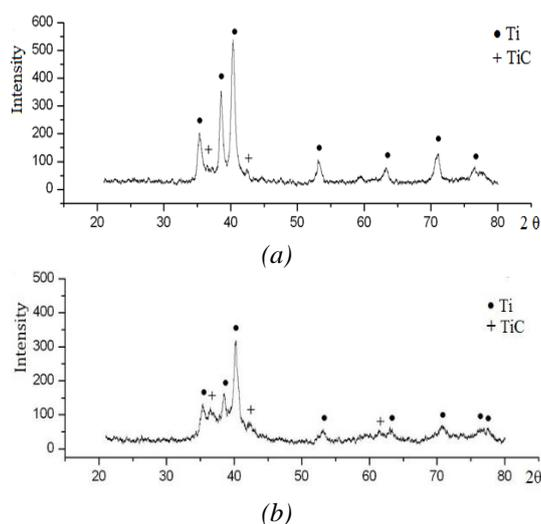
Figure 6. X-ray diffraction pattern of the mixture of Ti/ CNT after MA of different duration: 2 min (a), 4 min. (b).
