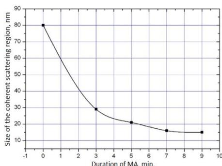
Fig. 8. Dependence of the value of the coherent scattering region of titanium on the MA duration of the Ti / CNT mixture.
