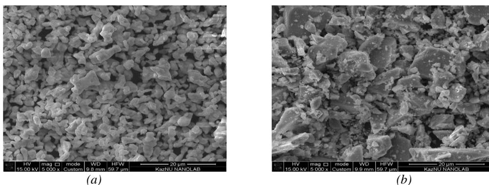
Fig. 1. SEM images of the initial components: a –  $\text{BaCrO}_4$ ; b –  $\text{TiB}_2$ .
