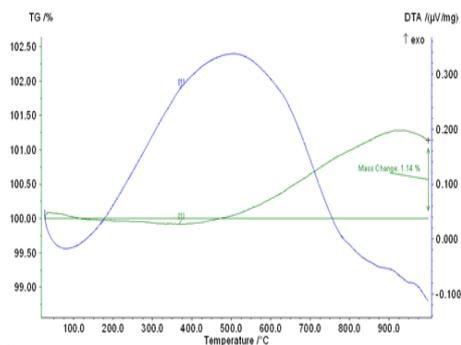
Fig. 9. Thermal analysis of the delay composition  $BaCrO_4$ -Ti/CNT.
