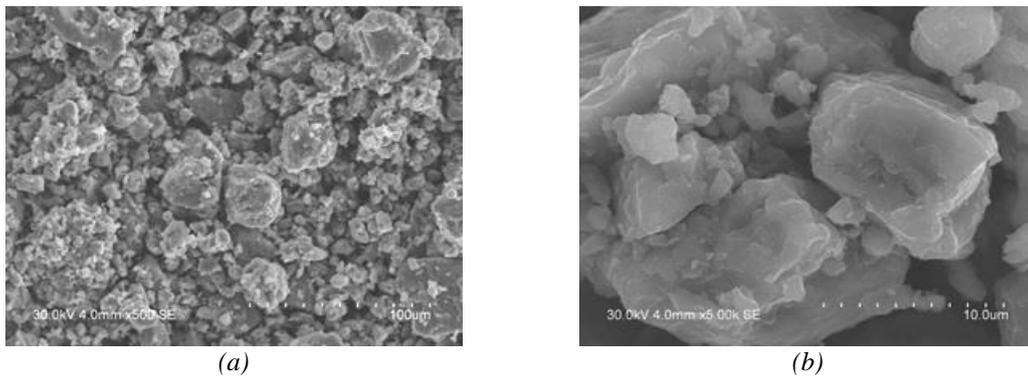
*Fig. 4. Micrographs of a Ti + 4% CNT sample after 8 min. MA: a – Ti + 4% CNT; b – the surface of an individual titanium particle.*
