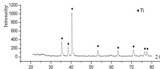
*Fig. 5. X-ray diffraction pattern of the initial mixture without MA.*
