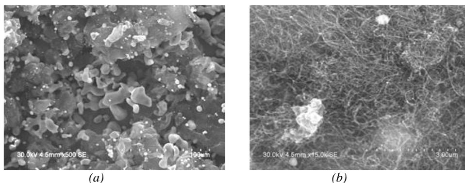
Fig. 2. Micrographs of the initial mixture: a – Ti + 4% CNT; b – the surface of an individual titanium particle.
