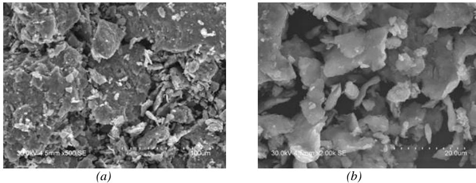
*Fig. 3. Micrographs of a Ti + 4% CNT sample after 2 min. MA: a – Ti + 4% CNT; b – the surface of an individual titanium particle.*
