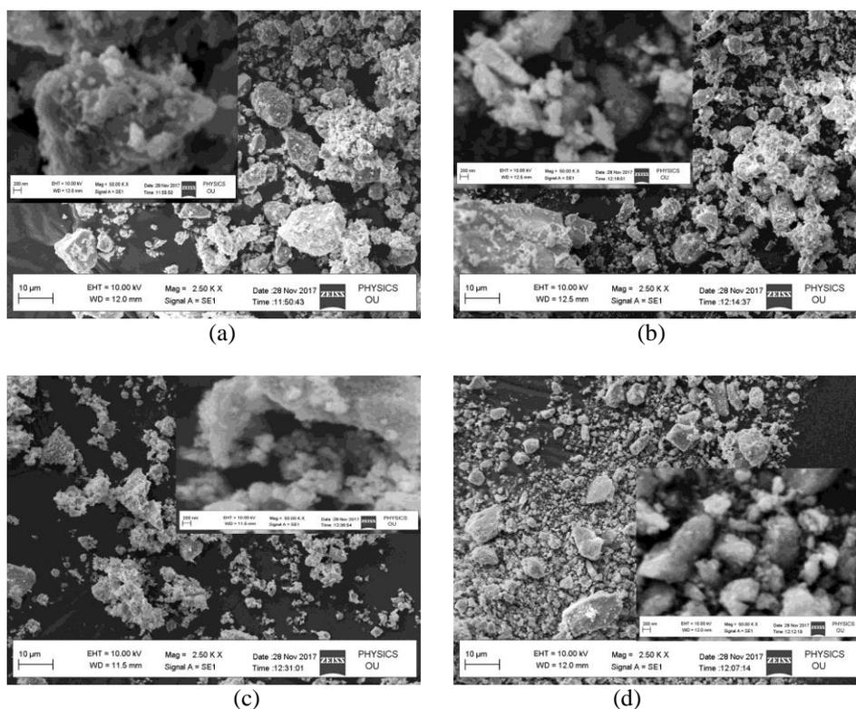
Fig. 2. Typical SEM patterns of the  $Zn_xFe_{2-x}O_3$  nanoparticles calcined at  $600^\circ C$  (a)  $x = 0$ , (b)  $x = 1$ , and calcined at  $800^\circ C$  (c)  $x = 0$  and (d)  $x = 1$ .
