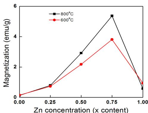
Fig. 5 Magnetization at 15 kOe of  $Zn_xFe_{2-x}O_3$  ( $x = 0$  to 1 with step of 0.25) nanoparticles prepared at 600°C and 800°C.
