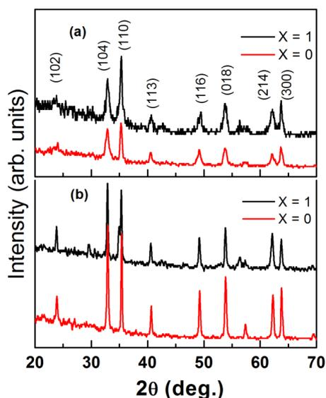
Fig. 1. Typical XRD patterns of the  $Zn_xFe_{2-x}O_3$  nanoparticles calcined at (a)  $600^\circ\text{C}$  and (b)  $800^\circ\text{C}$  temperatures.
