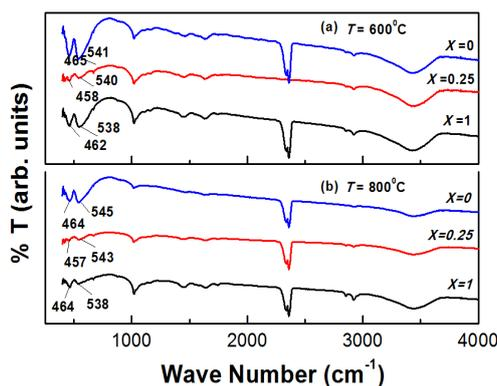
Fig. 3. FTIR spectrum for the  $Zn_xFe_{2-x}O_3$  nanoparticles prepared at (a) 600°C and (b) 800°C temperatures.
