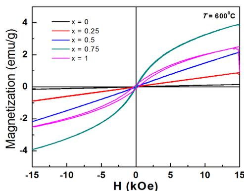
Fig. 4. Magnetic hysteresis curves of  $Zn_xFe_{2-x}O_3$  ( $x = 0$  to 1 with step of 0.25) nanoparticles prepared at 600°C.
