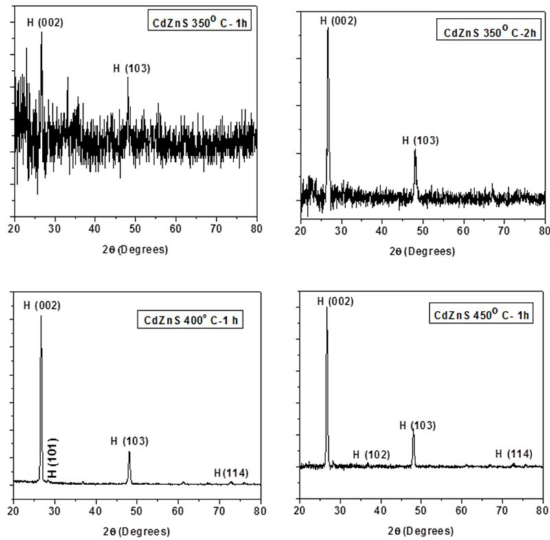
Fig. 1. XRD patterns of annealed CdZnS thin films.
