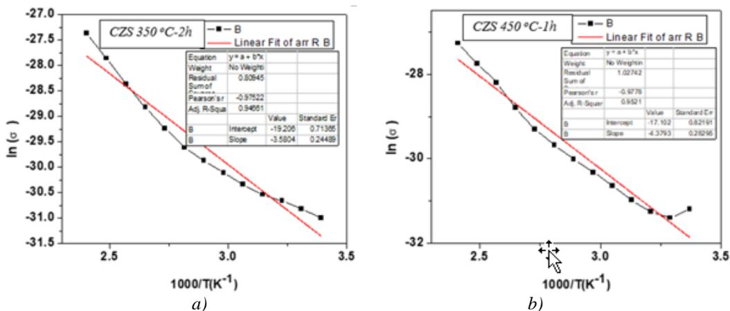
Fig. 4. Variation of  $\ln(\sigma)$  versus  $1000/T$  of (a) CZS 350 °C-2h (b) CZS 450 °C-1h.
