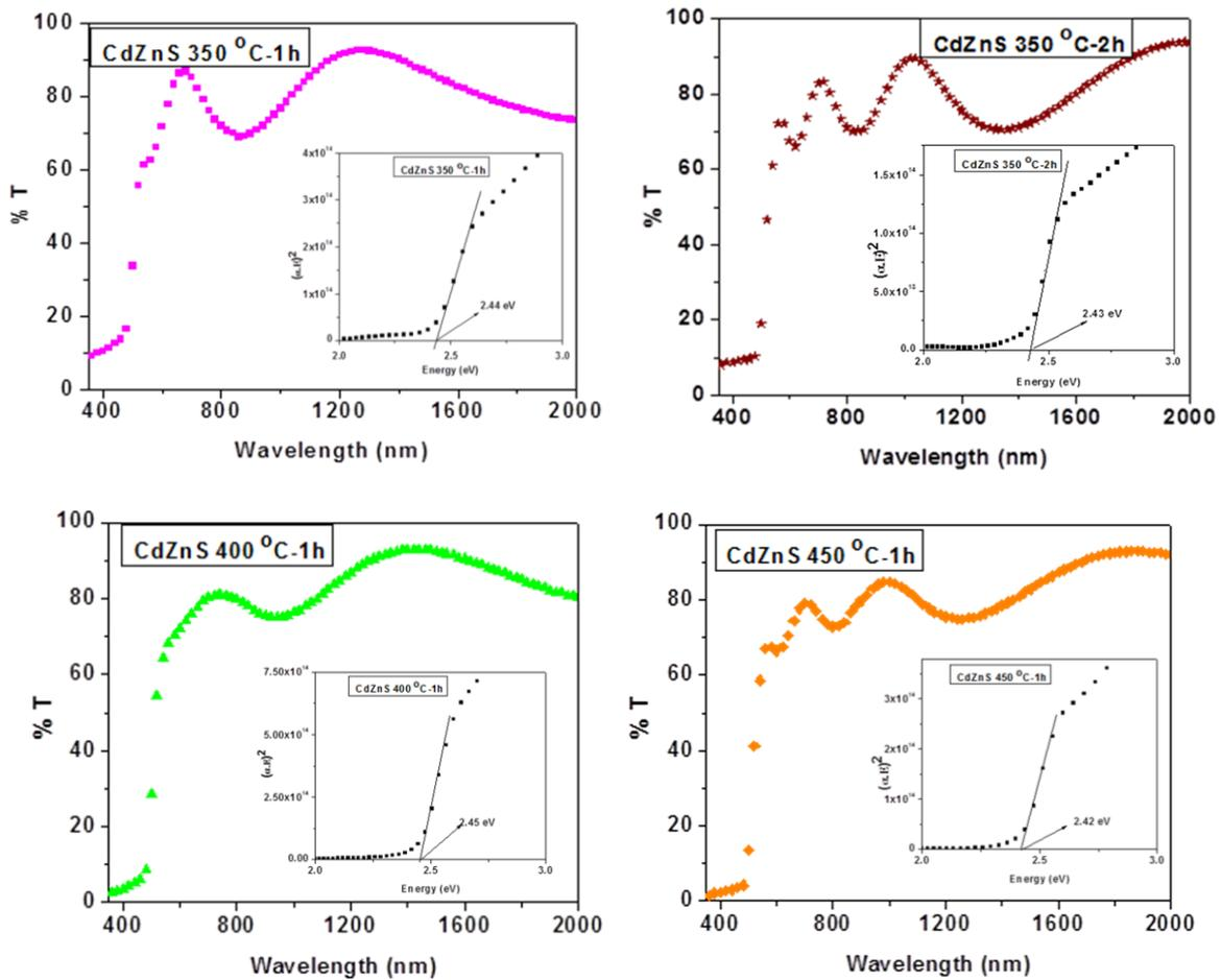
Fig. 3. Transmittance vs. Wavelength of different temperature annealed CdZnS thin film samples.
