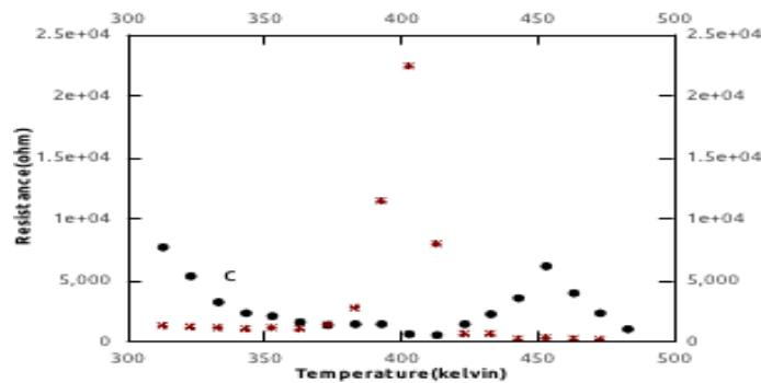
Fig 10(d) Variation of resistance with temperature of copper sulfide nanoparticles synthesized by Precipitation method.
