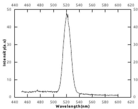
*Fig 7.P.L. spectrum of copper sulfide nanoparticles synthesized by solvothermal method.*
