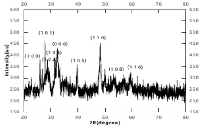
Fig 1(b) Indexed XRD pattern of CuS nanoparticles synthesized by precipitation method.
