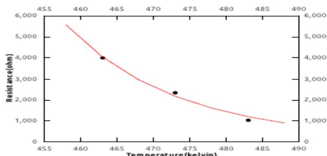
Fig 10(f) Variation of resistance with temperature inthe region 460K-490K.
