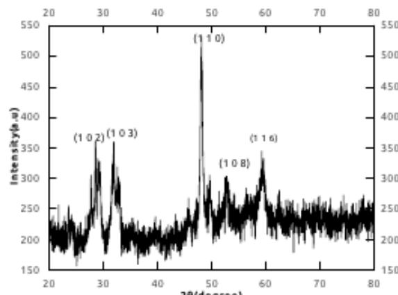
Fig 1(d) Indexed XRD pattern of CuS pellet synthesized by precipitation method. ( $\lambda=1.54 \text{ \AA}^0$ )
