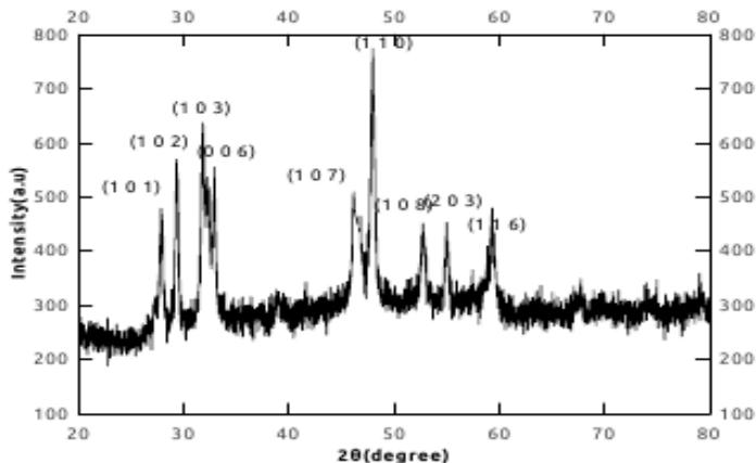
*Fig 1(a) Indexed XRD pattern of CuS nanoparticles synthesized by solvothermal method .*
