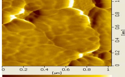
Fig 4. AFM image of copper sulfide nanoparticles synthesized by solvothermal method.
