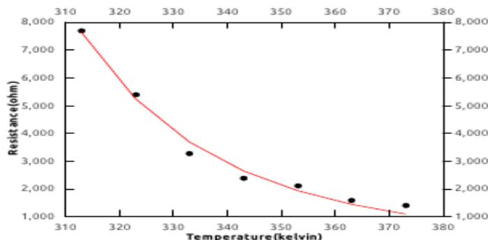
Fig 10(e) Variation of resistance with temperature inthe region 310K-398K.
