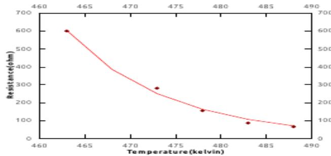
Fig 10(c) Variation of resistance with temperature inthe region 460K-490K.
