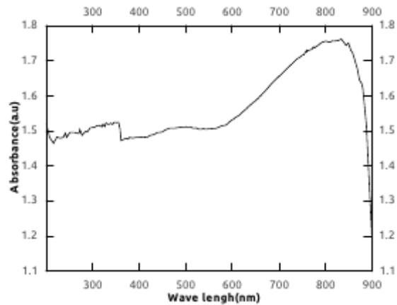
*Fig 5. Optical absorption spectrum of copper sulfide nanoparticles synthesized by solvothermal method.*
