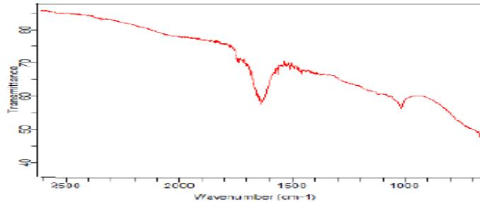
Fig 9 FTIR spectrum of copper sulfide nanoparticles synthesized by solvothermal method.
