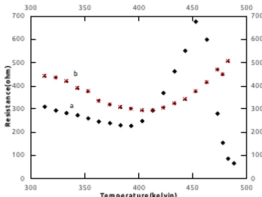
Fig 10(a) Variation of resistance with temperature of copper sulfide nanoparticles synthesized by solvothermal method.
