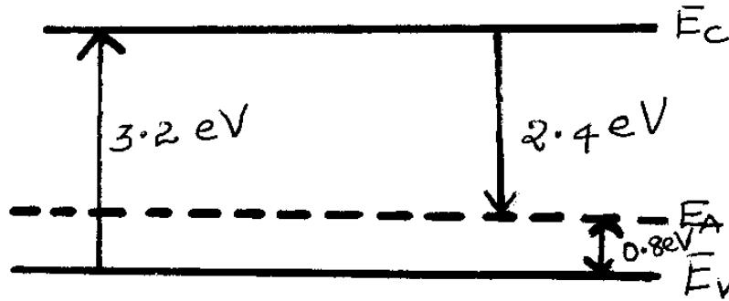
Fig 8 Emission absorption energy level diagram of copper sulfide nanoparticles synthesized by solvothermal method.
