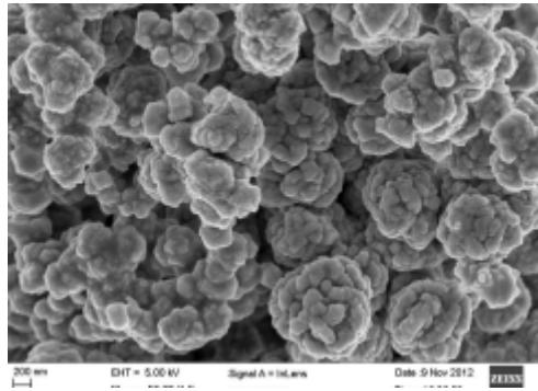
Fig 3. SEM image of copper sulfide nanoparticles synthesized by solvothermal method.
