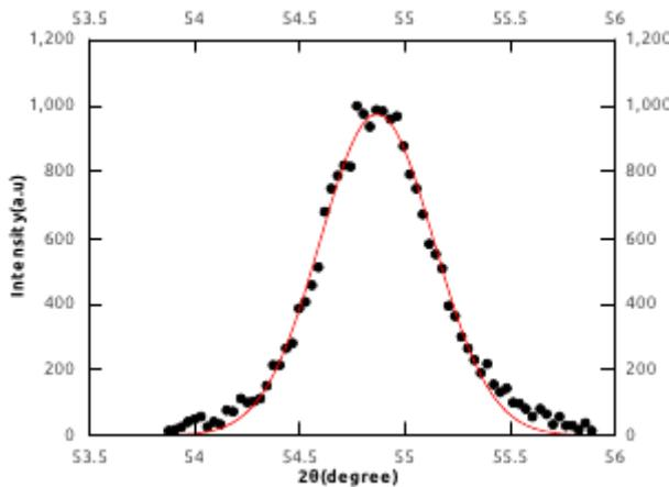
Fig 2. Gaussian fitted (1 1 0) peak of copper sulfide nanoparticles.
