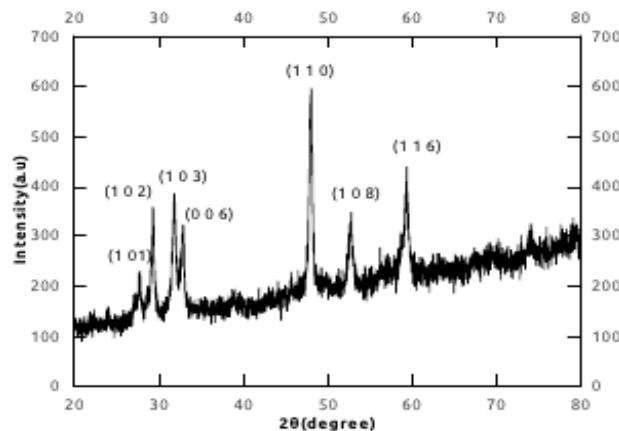
Fig 1(c) Indexed XRD pattern of CuS pellet synthesized by solvothermal method.
