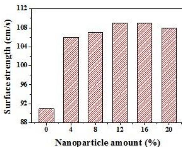
*Fig. 4. Influence of nanoparticle amount on surface strength of coated paper (Paper coating formulation: kaolin 80-96 %, the weight ratio (1:1) of  $\text{TiO}_2$  to  $\text{CaCO}_3$ . Based on the total weight of pigment, cationic starch 12 pph, HEC 0.4 pph, dispersant 0.6 pph. Solid content of paper coatings 55 wt%)*
