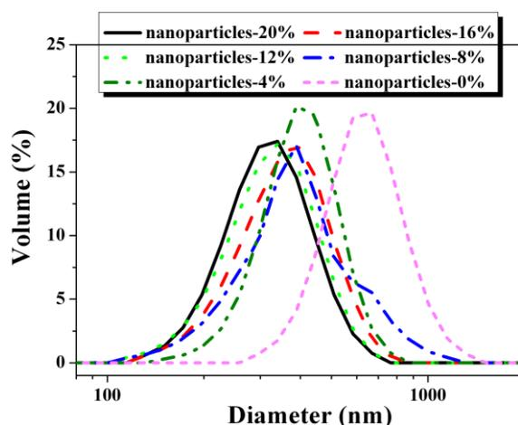
Fig. 3. Influence of nanoparticle amount on particle size distribution of paper coatings (Paper coating formulation: kaolin 80-96 %, the weight ratio (1:1) of  $\text{TiO}_2$  to  $\text{CaCO}_3$ . Based on the total weight of pigment, cationic starch 12 pph, HEC 0.4 pph, dispersant 0.6 pph. Solid content of paper coatings 55 wt%)
