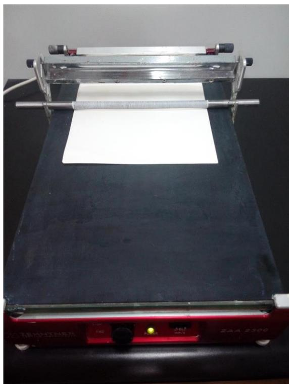
*Fig. 1. Surface application configuration of paper coatings onto cellulosic paper*
