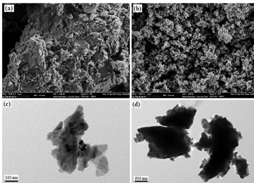
Fig. 2. SEM images of (a) kaolin, (b)  $\text{TiO}_2$  nanoparticles; TEM images of (c) and (d)  $\text{CaCO}_3$  nanoparticles with different magnification
