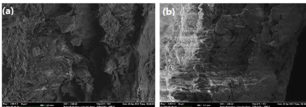
*Fig. 8. SEM images of cross-sections of coated paper: (a) coated paper formed from paper coating without nanoparticles; (b) coated paper formed from paper coatings with 4% nanoparticle pigments.*
