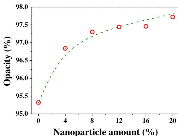
Fig. 6. Influence of nanoparticle amount on opacity of coated paper (Paper coating formulation: kaolin 80-96 %, the weight ratio (1:1) of  $\text{TiO}_2$  to  $\text{CaCO}_3$ . Based on the total weight of pigment, cationic starch 12 pph, HEC 0.4 pph, dispersant 0.6 pph. Solid content of paper coatings 55 wt%)
