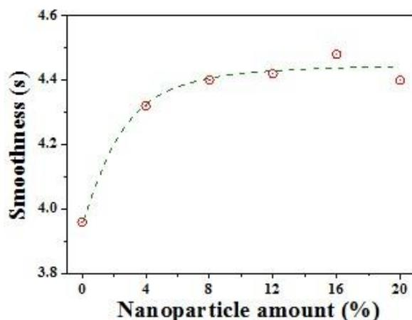
Fig. 5. Influence of nanoparticle amount on smoothness of coated paper
