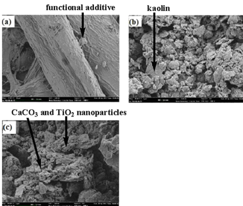
Fig. 7. SEM images of uncoated and coated paper surface: (a) uncoated paper; (b) coated paper formed from paper coatings without nanoparticles; (c) coated paper from paper coatings with 4% nanoparticle pigments.
