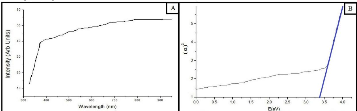
Fig. 1[a].Transmission spectra of (Cd,Zn)S:Ag;[b].Square of the absorption co-efficient with Photon energy of (Cd,Zn)S:Ag
