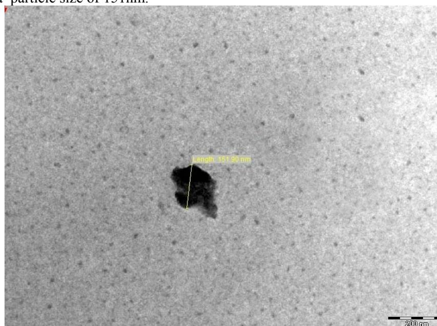
Fig. 5. TEM result of the  $(\text{Cd,Zn})\text{S:Ag}$
