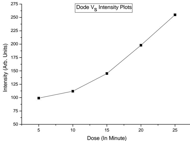
Fig. 7. Dose Vs Intensity plot of (Cd,Zn)S:Ag phosphor
