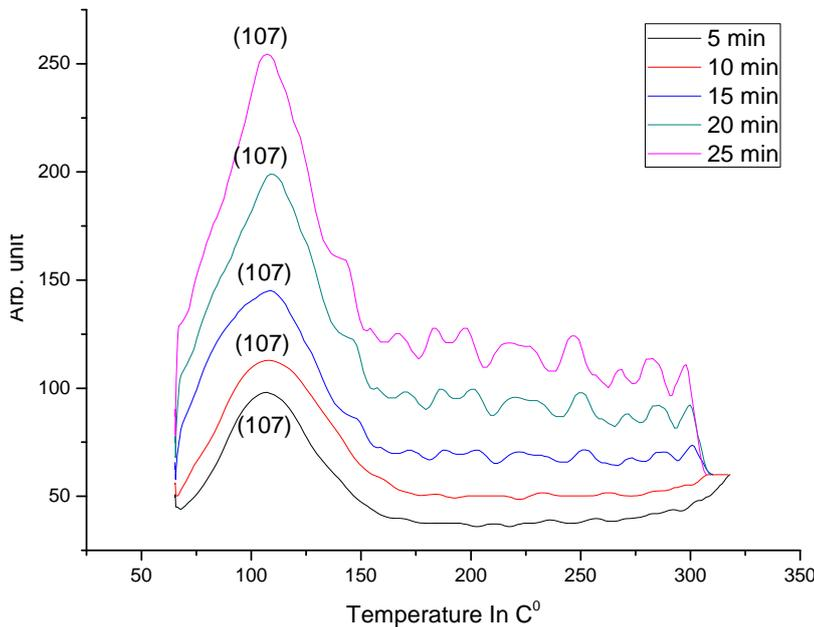
Fig. 6. TL Glow curve of (Cd,Zn)S:Ag phosphor
