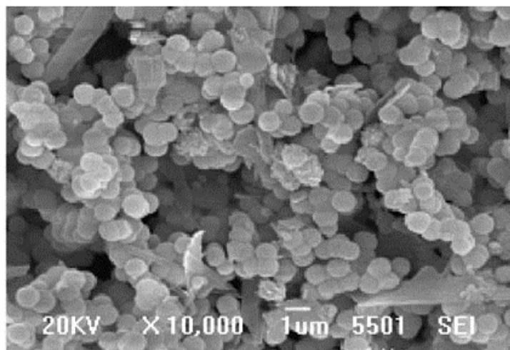
Fig. 3. SEM image of (Cd,Zn)S:Ag
