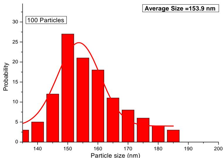
Fig. 4. Histogram of particle size distribution for the studied  $(\text{Cd,ZnS})\text{:Ag}$  phosphors
