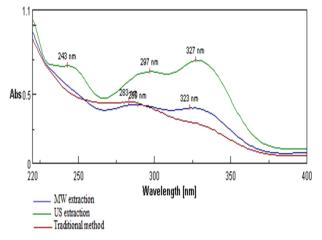
Fig. 1. UV-Vis spectra for methanolic extracts
