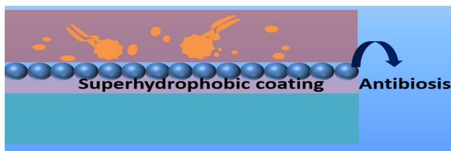
Fig. 13. Schematic of antimicrobial mechanism of PTFE@TiO<sub>2</sub>/epoxy superhydrophobic coating.
