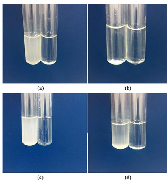
*Fig. 5. Suspended photographs of the samples before and after surface modification with water:(a)-PLNPs Suspension photos,(b)-The photos of PLNPs suspension after standing, (c)-SiO<sub>2</sub>-PLNPs Suspension photos, (d)-The photos of SiO<sub>2</sub>-PLNPs suspension after standing.*
