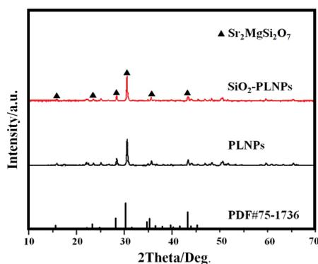
Fig. 1. The XRD patterns of PLNPs and SiO<sub>2</sub>-PLNPs.
