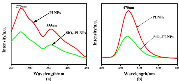
Fig. 3. The excitation spectra (a) and the emission spectra (b) of the PLNPs and SiO<sub>2</sub>-PLNPs.
