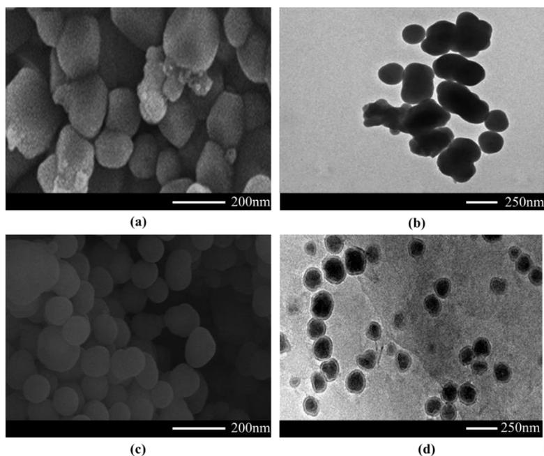
Fig. 2. (a) SEM images of PLNPs (b) TEM images of PLNPs (c) SEM images of SiO<sub>2</sub>-PLNPs, (d) TEM images of SiO<sub>2</sub>-PLNPs.
