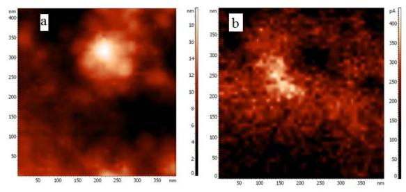
Fig.10. AFM(a) u MFM(b) images of nanocomposite  $PE+Fe_3O_4$ .
