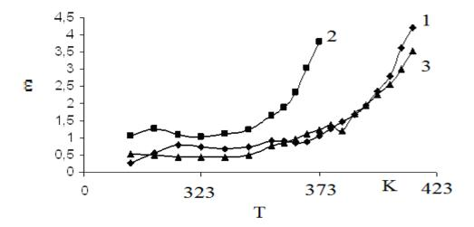
Fig.3. Dependence of permittivity of nanocomposite from temperature 1. PE+5 ml  $Fe_3O_4$ , 2. PE+10 ml  $Fe_3O_4$ , 3.PE+15ml  $Fe_3O_4$ ,
