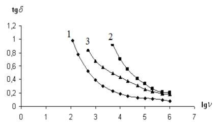
*Fig.5. Dependence of dielectric loss tangent from frequency for nanocomposites PE+Fe<sub>3</sub>O<sub>4</sub>: 1.PE+5% Fe<sub>3</sub>O<sub>4</sub>, 2. PE+10% Fe<sub>3</sub>O<sub>4</sub>, 3. PE+15% Fe<sub>3</sub>O<sub>4</sub>*
