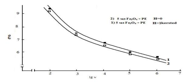
Fig.8 Dependence of permittivity from frequency of measurement of nanocomposite  $PE+5\%Fe_3O_4$  before and after polarization in magnetic field.
