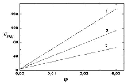
Fig. 2 The dependence of permittivity of nanocomposites from concentration of nanomagnetite.  $H=4,1\cdot10^{5} A/M-1, H=0 \text{ and } H=2,7\cdot10^{5} A/M-2, H=1,3\cdot10^{5} A/M-3.$
