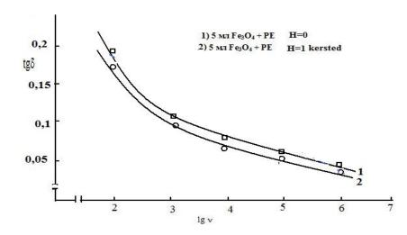
Fig.7 Dependence of dielectric loss tangent from frequency of measurement of nanocomposite PE+5%Fe<sub>3</sub>O<sub>4</sub> before and after polarization in magnetic field.
