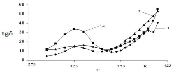
Fig.4 Dependence of dielectric loss tangent from temperature for nanocomposite 1. PE+5 ml  $Fe_3O_4$ , 2. PE+10 ml  $Fe_3O_4$ , 3.PE+15ml  $Fe_3O_4$
