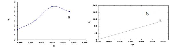
Fig.1 Dependence of permittivity of nanocomposite  $PE+Fe_3O_4$  from concentration: a) experimental, b) theoretical
