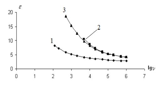
Fig.6. Dependence of permittivity from frequency for nanocomposites PE+ Fe<sub>3</sub>O<sub>4</sub>: 1.PE+5% Fe<sub>3</sub>O<sub>4</sub>, 2. PE+10% Fe<sub>3</sub>O<sub>4</sub>, 3. PE+15% Fe<sub>3</sub>O<sub>4</sub>
