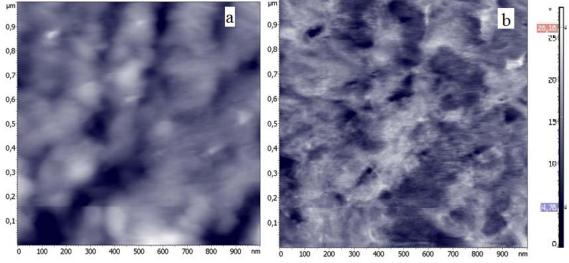
Fig.9 AFM image of nanocomposite surface  $PE + Fe_3O_4$ a) Before treatment in constant magnetic field, b) after polarization in constant magnetic field
