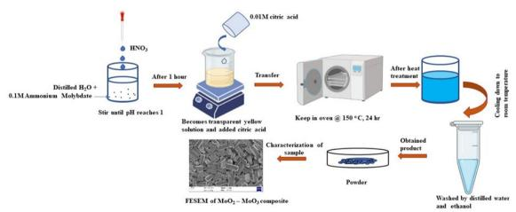
Fig. 1. Schematic representation for the synthesis of  $MoO_3 - MoO_2$  composite.
