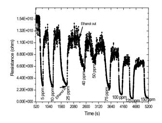
Fig. 6. Response – Recovery characteristics of MoO<sub>3</sub> – MoO<sub>2</sub> composite.
