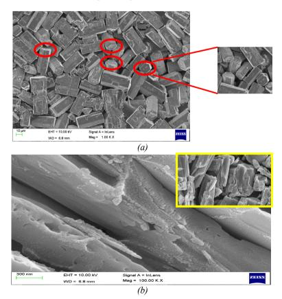
Fig. 4. FE-SEM image of MoO<sub>3</sub> – MoO<sub>2</sub> composite under (a) lower magnification (inset: hexagonal facets) and (b) higher magnification.
