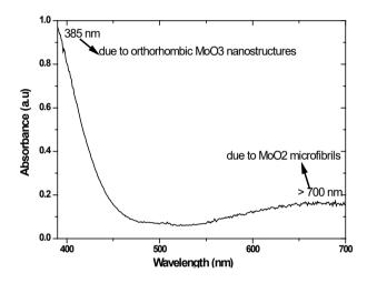
Fig. 5. UV - V is absorption spectra of  $MoO_3 - MoO_2$  composite under (a) lower magnification (inset: hexagonal facets) and (b) higher magnification.
