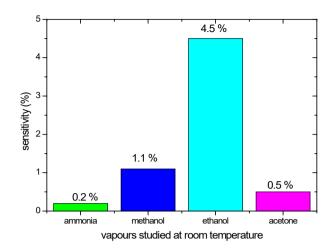
Fig. 7. Selectivity amidst various volatile vapours by  $MoO_3 - MoO_2$  composite.
