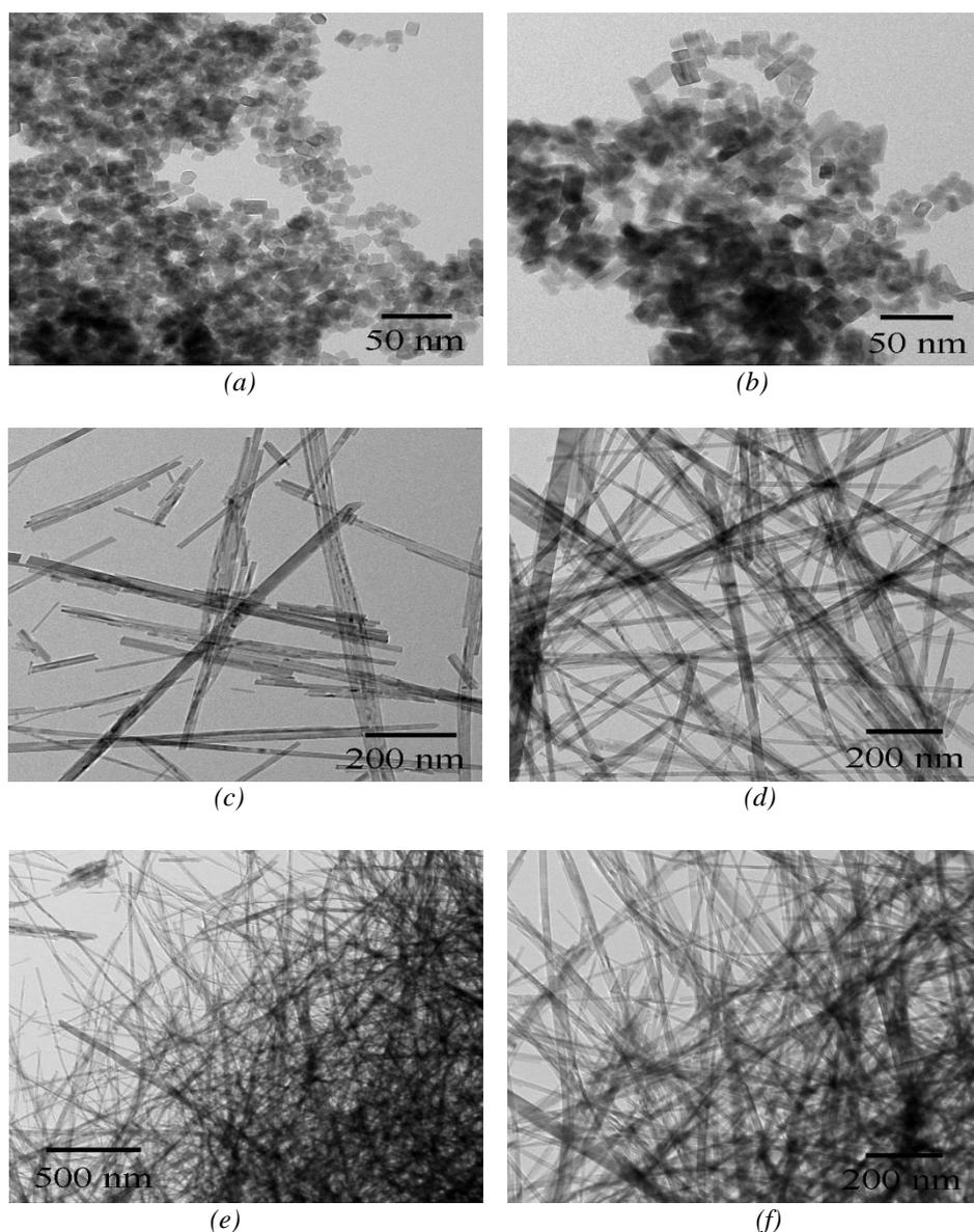
*Fig. 3. TEM images of the as-synthesized CdS products synthesized by reflux at (a) 60 °C and (b) 80 °C for 2 h, and reflux-assisted solvothermal method at (c) 120 °C for 12 h, (d) 160 °C for 12 h and (e, f) 160 °C for 24 h.*
