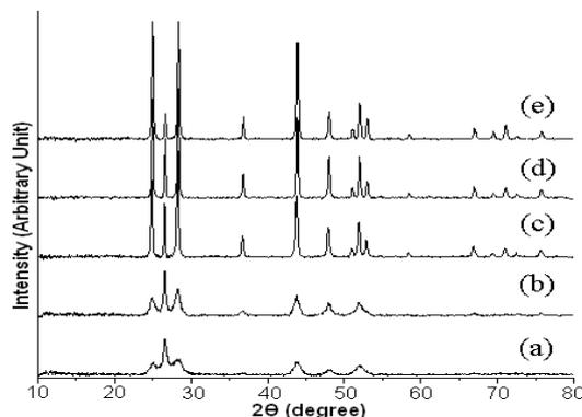
Fig. 1. XRD patterns of the as-synthesized CdS products synthesized by reflux at (a) 60 °C and (b) 80 °C for 2 h, and reflux-assisted solvothermal method at (c) 120 °C for 12 h, (d) 160 °C for 12 h and (e) 160 °C for 24 h.
