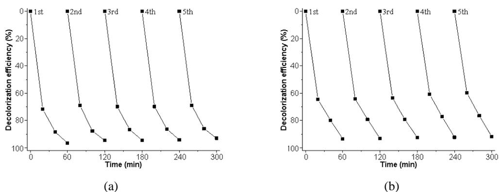
Fig. 7. Recyclability of CdS nanowires for photodegradation of (a) MO and (b) RhB under visible light irradiation.
