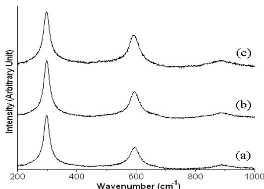
Fig. 2. Raman spectra of CdS nanowires synthesized by reflux-assisted solvothermal method at (a) 120 °C for 12 h, (b) 160 °C for 12 h and (c) 160 °C for 24 h.
