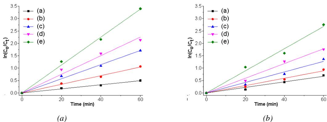
Fig. 6. Pseudo-first order plots for (A) MO and (B) RhB photodegradation in the solutions containing as-synthesized CdS products synthesized by reflux method at (a) 60 °C and (b) 80 °C for 2 h, and reflux-assisted solvothermal method at (c) 120 °C for 12 h, (d) 160 °C for 12 h and (e) 160 °C for 24 h.
