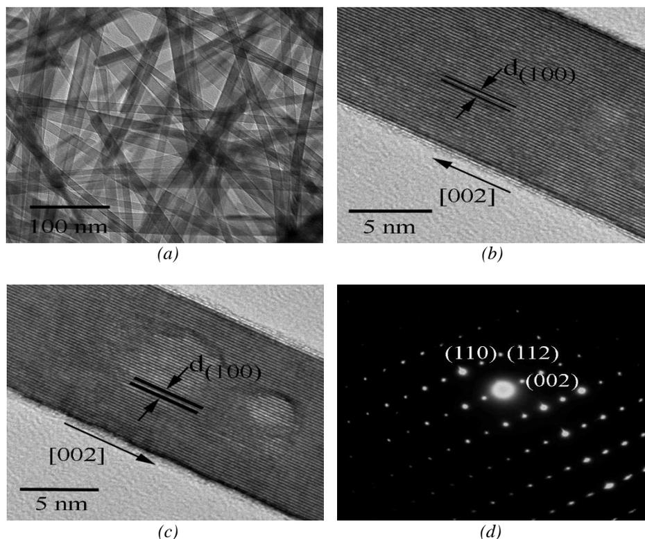
Fig. 4. TEM and HRTEM images, and SAED pattern of CdS nanowires synthesized by reflux-assisted solvothermal method at 160 °C for 24 h.
