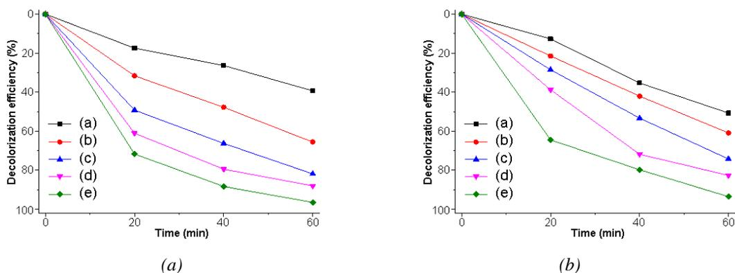
Fig. 5. Decolorization efficiency of (A) MO and (B) RhB in the solutions containing as-synthesized CdS products synthesized by reflux at (a) 60 °C and (b) 80 °C for 2 h, and reflux-assisted solvothermal method at (c) 120 °C for 12 h, (d) 160 °C for 12 h and (e) 160 °C for 24 h.
