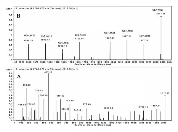
Fig. 1. A.MS/MS spectrum of  $[TABCD]^+$  fragmentation energy  $E_{LAB}=20 \text{ eV}$ ; B. detailed view m/z span [1500-2050]
