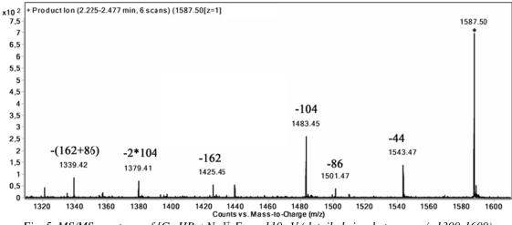
Fig. 5. MS/MS spectrum of  $[G_7-HB_5+Na]^+ E_{LAB}=110 \text{ eV}$  (detailed view between m/z 1300-1600)
