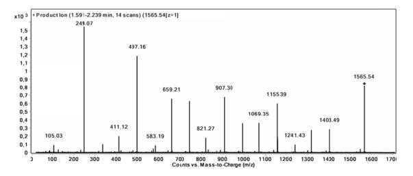
Fig. 4. MS/MS spectrum of  $[HB_5-CD_7]^+ E_{LAB}=15 \text{ eV}$
