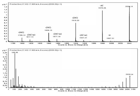
Fig. 2. MS/MS spectrum of  $[TABCD+Na]^+ E_{LAB}=120 \text{ eV}$ : A. full spectrum; B. detailed spectrum in the region m/z = [1780 - 2060]
