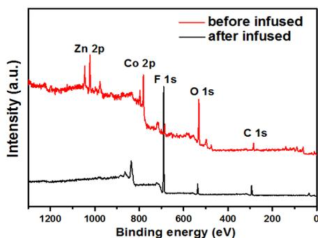
Fig. 4. XPS spectra of before and after infused lubricant oil.
