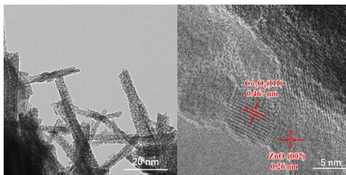
Fig. 2. (a) TEM images and (b) HRTEM images of cluster-like  $\text{ZnO}@Co_3O_4$ .
