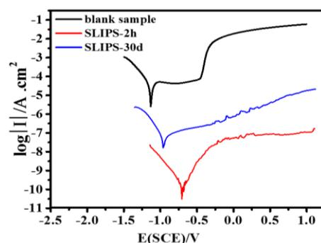
Fig. 6. Polarization curves of different samples immersed in 3.5 wt% NaCl solution.
