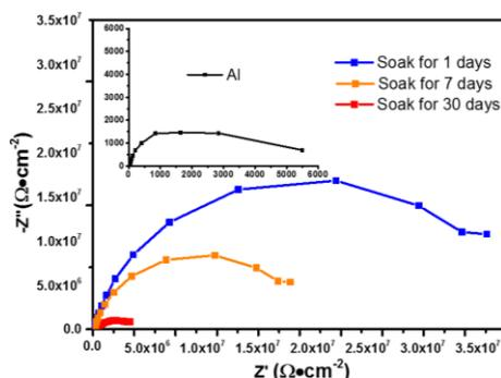
Fig. 7. EIS results of SLIPS based on cluster-like  $\text{ZnO}@ \text{Co}_3\text{O}_4$  after immersion in a 5% NaCl solution for different times.
