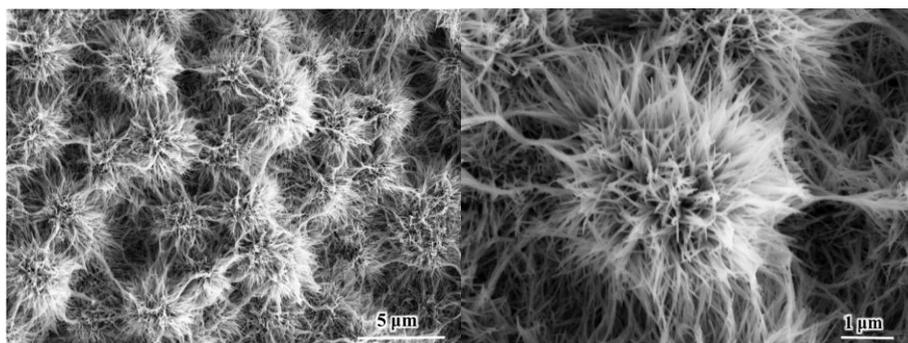
Fig. 1. SEM images of (a) low magnification and (b) high magnification of cluster-like  $\text{ZnO}@Co_3O_4$ .
