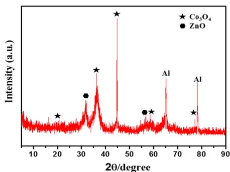
Fig. 3. XRD pattern of cluster-like  $\text{ZnO}@Co_3O_4$ .
