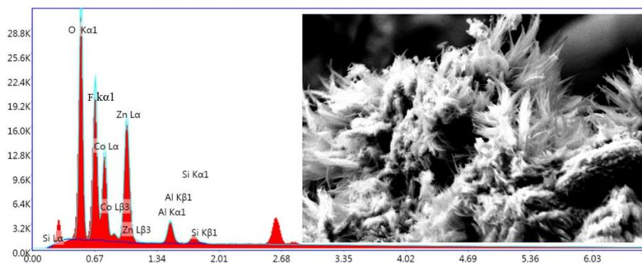
Fig. 8. SEM and EDS images of SLIPS based on cluster-like  $\text{ZnO}@Co_3O_4$  after 30 d immersion.
