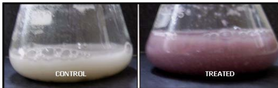
Fig 2 F. oxysporum 284 biomass before (control) and after treatment (treated) with 1mM gold hypochlorite solution for the period of 72 hrs.
