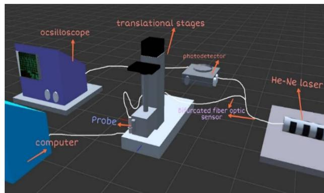
*Fig. 1. 3D schematic diagram of the FODS system.*
