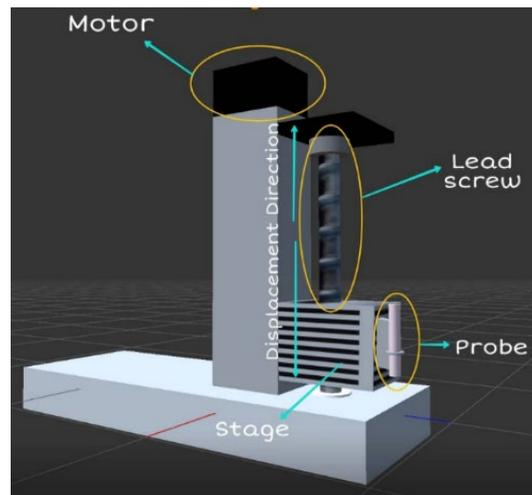
*Fig. 2. 3D schematic diagram of the linear translational stage.*
