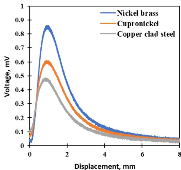
*Fig. 4. Voltage against displacement for different metal samples.*
