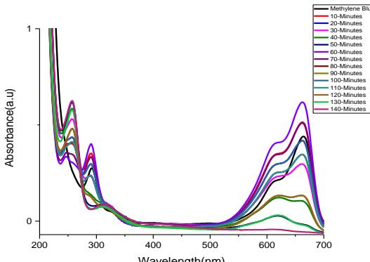
Fig. 11. Photodegradation of Ag/Chitosan with 3mL Acetic acid.
