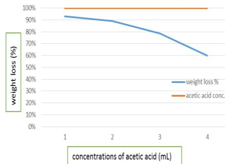
*Fig. 13. Weight loss of paper with increasing Acetic acid concentration.*
