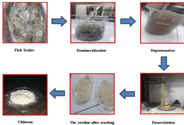
*Fig. 1. Flowsheet diagram showing extraction of Chitosan.*
