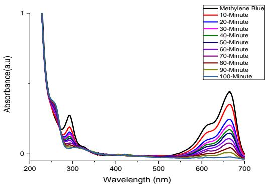
*Fig. 8. Photodegradation of chitosan with 3mL Acetic acid.*
