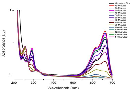
*Fig. 9. Photodegradation of Ag/chitosan with 5mL Acetic acid.*
