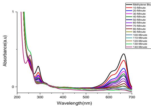
Fig. 10. Photodegradation of Ag/Chitosan with 4mL Acetic acid.
