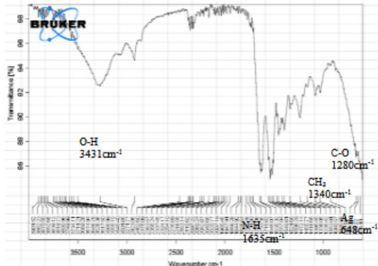
Fig. 5. FTIR spectrum of Ag/Chitosan
