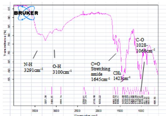
*Fig. 4. FTIR spectrum of Chitosan.*
