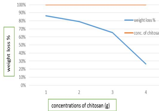
*Fig. 12. Weight loss of paper with increasing Chitosan concentration.*
