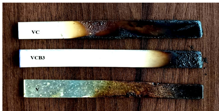
Fig. 4. Burned test specimens of V, VC and VCB3 composite samples.
