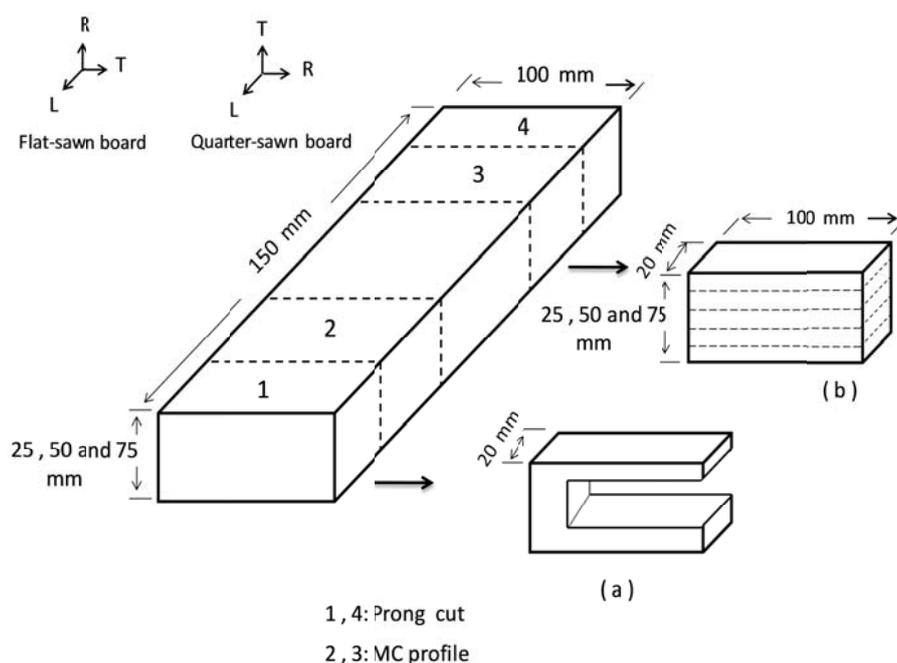
Fig. 1. A schematic of sample cut for measurements of drying stresses (a), and MC profiles (b) of the dried boards.
