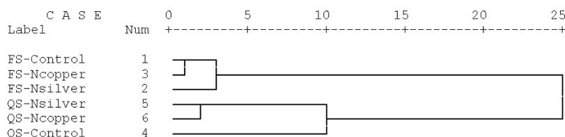
Fig. 4. Cluster analysis of 75-mm-boards based on drying rate above FSP, drying rate below FSP, MC gradient slope, and drying stress (FS=Flat-sawn; QS=Quarter-sawn)
