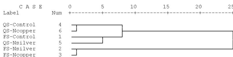
Fig. 3. Cluster analysis of 50-mm-boards based on drying rate above FSP, drying rate below FSP, MC gradient slope, and drying stress (FS=Flat-sawn; QS=Quarter-sawn)
