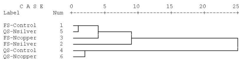
Fig. 2. Cluster analysis of 25-mm-boards based on drying rate above FSP, drying rate below FSP, MC gradient slope, and drying stress (FS=Flat-sawn; QS=Quarter-sawn)
