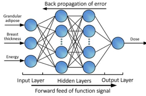
Fig. 4 Neural Network architecture of the designed model
