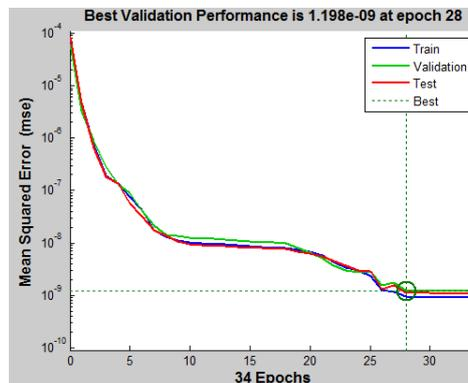
Fig. 5. The output of MSE variation throughout the ANN model generating process
