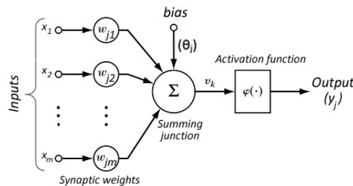
Fig. 3 Artificial neuron structure
