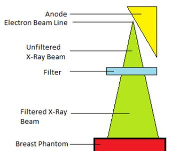
*Fig. 2. Total simulation geometry*
