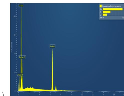
Fig. 4. ED pattern of HC@Fe<sub>3</sub>O<sub>4</sub>
