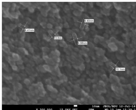
Fig. 3. SEM image of HC@Fe<sub>3</sub>O<sub>4</sub>
