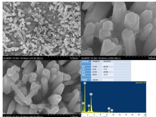
Fig. 2e. FESEM images of various magnification rates and EDS analysis of the ZnS/ZnO core-shell nanostructures with deposition time of (e) 20 mins.
