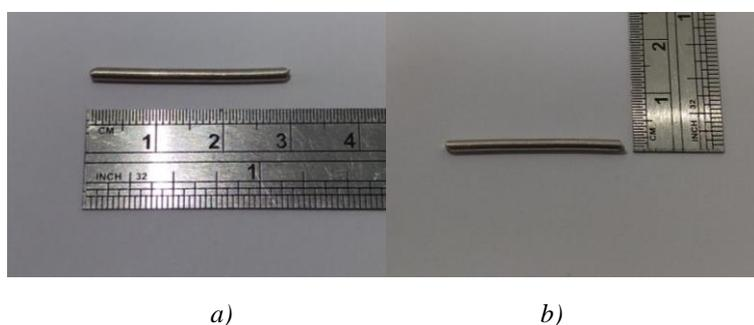
Fig. 1. Photos of a silver wire with (a) 3 cm length and (b) 2 mm diameter.
