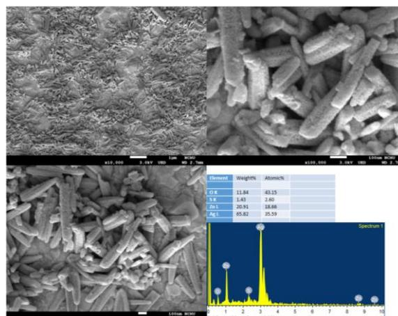
Fig. 2c. FESEM images of various magnification rates and EDS analysis of the ZnS/ZnO core-shell nanostructures with deposition time of (c) 10 mins
