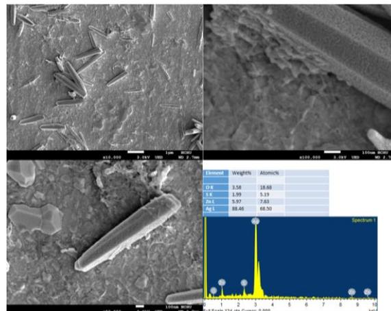
Fig. 2b. FESEM images of various magnification rates and EDS analysis of the ZnS/ZnO core-shell nanostructures with deposition time of (b) 5 mins
