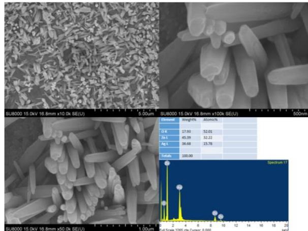
Fig. 2a. FESEM images of various magnification rates and EDS analysis of the ZnS/ZnO core-shell nanostructures with deposition time of (a) 0 min
