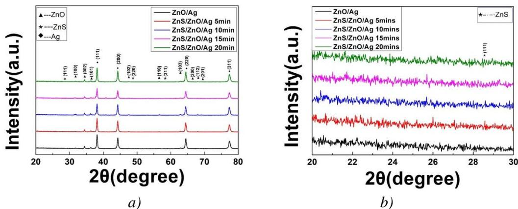
Fig. 3.(a) 20-80° XRD patterns of the ZnS/ZnO/silver wires with various ZnS deposition time (b) 20-30° XRD patterns of the ZnS/ZnO/silver wires with various ZnS deposition time
