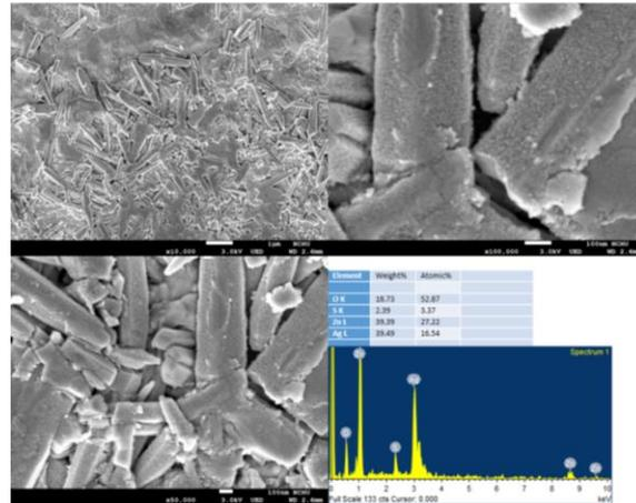
Fig. 2d. FESEM images of various magnification rates and EDS analysis of the ZnS/ZnO core-shell nanostructures with deposition time of (d) 15 mins
