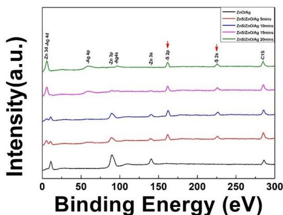
Fig. 4. XPS measurements of ZnS/ZnO/silver wires with various ZnS deposition time.
