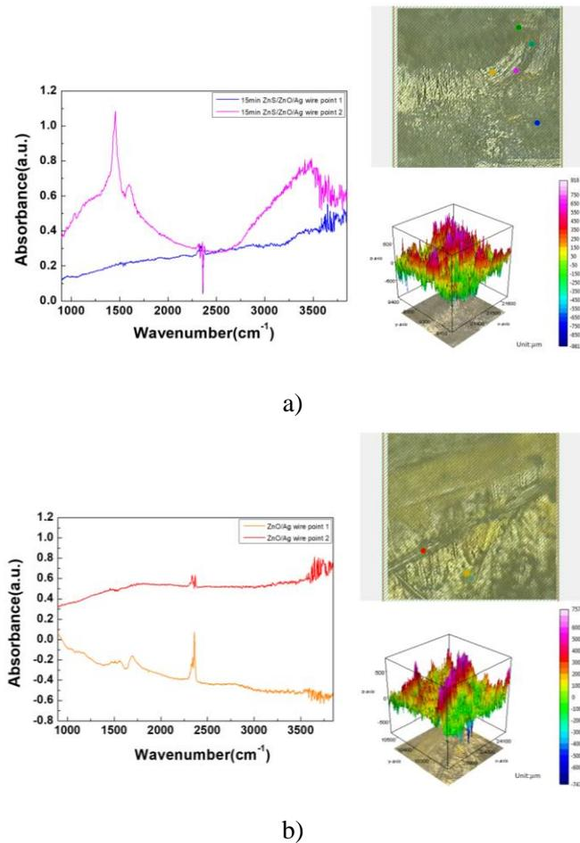
Fig. 5. FTIR measurement of (a) a ZnS/ZnO/silver wire and (b) a ZnO/silver wire.
