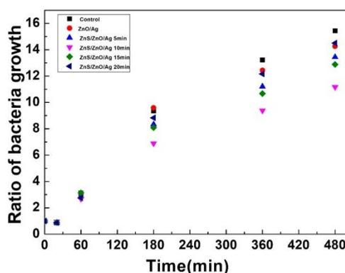
Fig. 6. OD 600 antibacterial tests for the ZnS/ZnO/silver wires with various ZnS deposition time
