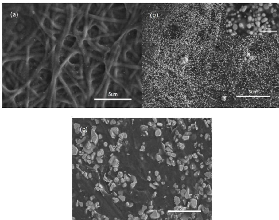
*Fig. 3. SEM images of Ag@PVA/CS substrates with different adsorption times:(a) 10min (b)20min (c)30min.*
