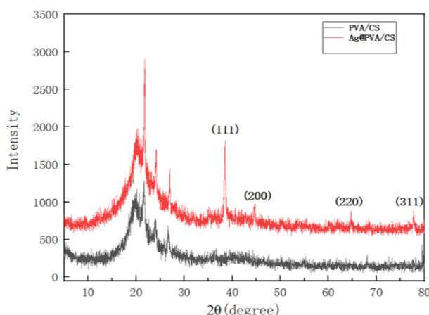
Fig. 4. XRD patterns of PVA/CS and Ag@PVA/CS substrates.
