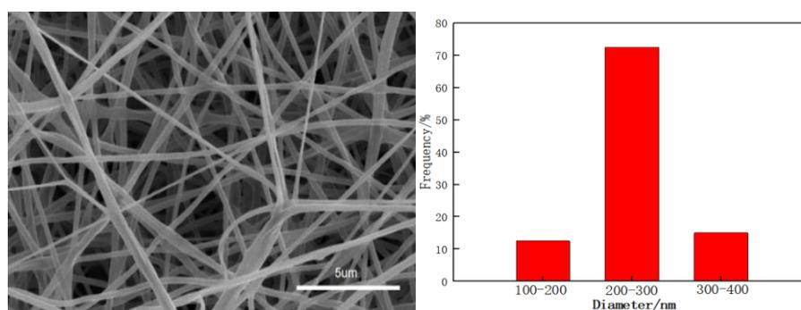
Fig. 1. (a) SEM image of PVA/CS nanofibers; (b) the diameter distribution of nanofibers.
