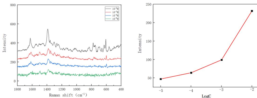
Fig. 7. (a) SERS spectra of Ag@PVA/CS substrates with different norfloxacin concentrations (b) peak intensity of  $1389\text{ cm}^{-1}$  in different SERS spectra in (a).
