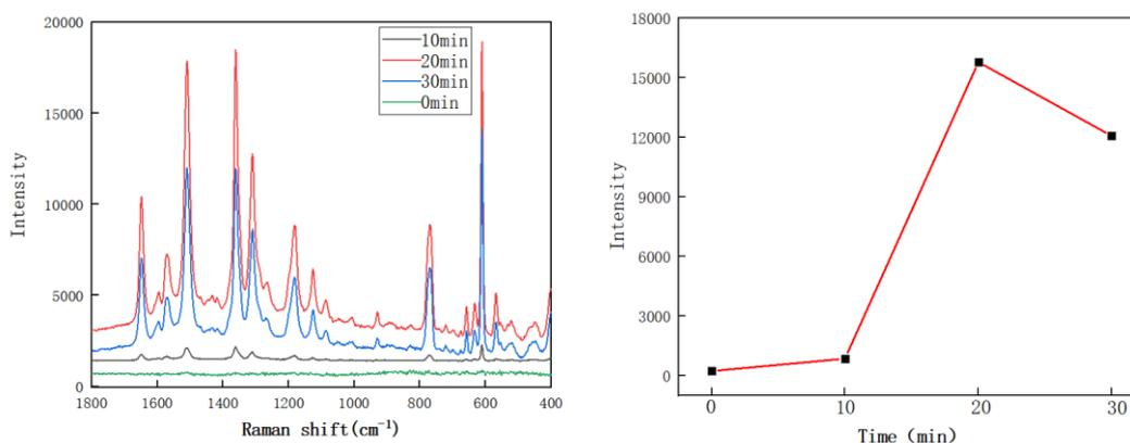
Fig. 5. (a) SERS spectra of Ag@PVA/CS substrates with different adsorption times (b) peak intensity of  $610\text{ cm}^{-1}$  in different SERS spectra in (a).
