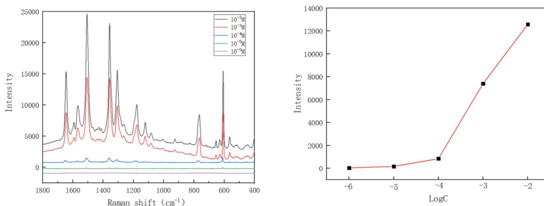
Fig. 6. (a) SERS spectra of Ag@PVA/CS substrates with different R6G concentrations (b) peak intensity of  $610\text{ cm}^{-1}$  in different SERS spectra in (a).
